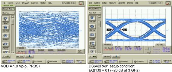
EQ[1:0] = 01 (~20 dB at 3 GHz) DEM[1:0] = 01 (-2 dB with VOD = 1.2 Vp-p)
