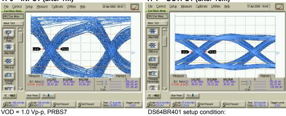
EQ[1:0] = 11 (~5.8 dB at 3 GHz) DEM[1:0] = F1 (-12 dB with VOD = 1.4 Vp-p)
