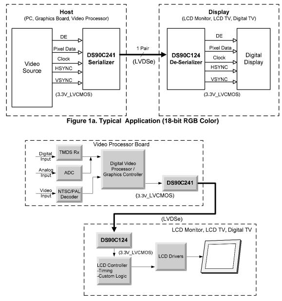
Figure 1b. Typical DS90C241/124 SERDES System Diagram
