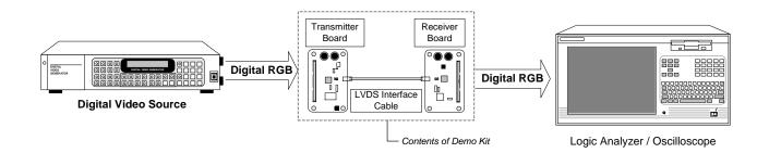
Figure 5. Typical SERDES Test Setup for Evaluation
