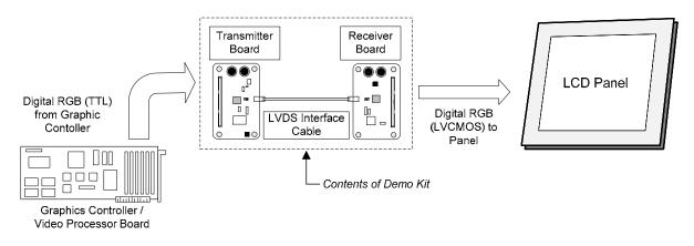
Figure 4. Typical SERDES Setup of LCD Panel Application
