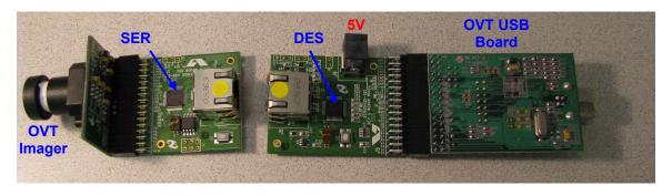
Figure 1. Imager - Serializer and Deserializer - Controller Connections
