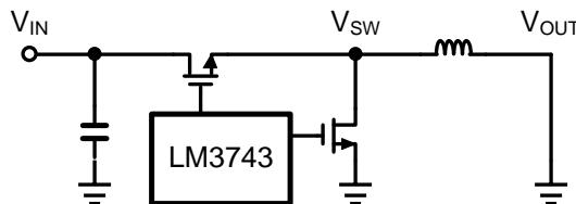
**Figure 3. Output Short-Circuit to Ground**
