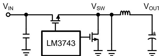
**Figure 4. Switch Node Short-Circuit to Ground**
