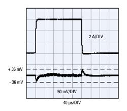
Figure 4. 2% Accurate Device with 940 µF of Output Capacitance
