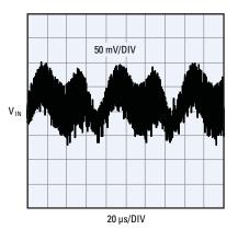
Figure 10. Two Independent Internal Oscillators, Not Synchronized
