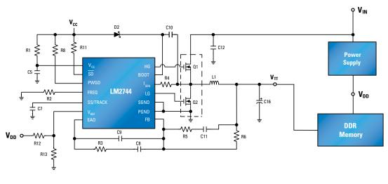
Figure 8. Typical DDR2 Application Circuit
