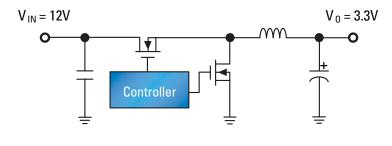
Figure 1. Simplified Buck Controller Circuit
