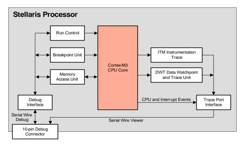
Figure 1. Debug and Trace Components in Stellaris Cortex-M3 Microcontrollers
