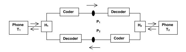
The analog signals, generated by either of the devices  $T_1$  and  $T_2$ , are at first conveyed by a short-distance, bidirectional, analog twowire line. The analog signals are then separated by the proper hybrid circuit ( $H_1$ ,  $H_2$ ), filtered using a band-pass filter with cutoff frequencies equal to 0 and 4 kHz to avoid aliasing, sampled at  $F_s = 8$  kHz, and quantified by a uniform 13 bit or 14 bit quantifier.
