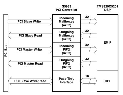
Figure 3. Data Paths of the S5933 PCI Controller/TMS320C6201 DSP Interface
