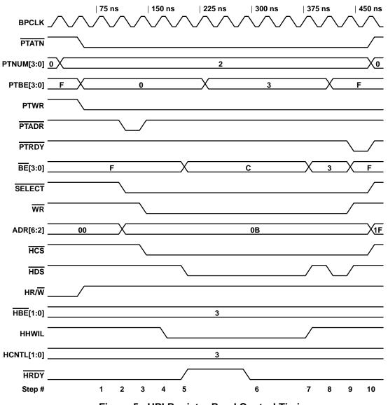
Figure 5. HPI Register Read Control Timing
