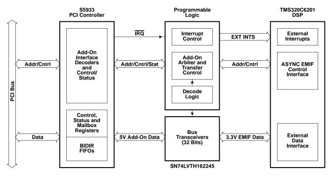
Figure 7. DSP EMIF Interface to the S5933 PCI Controller
