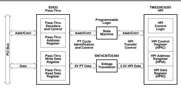
Figure 4. DSP HPI Interface to the S5933 PCI Controller
