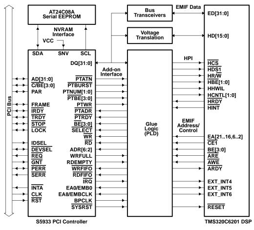
Figure 1. TMS320C6201 Interface to the S5933 PCI Controller
