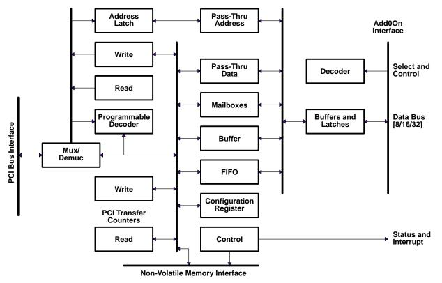
Figure 2. S5933 PCI Controller Block Diagram
