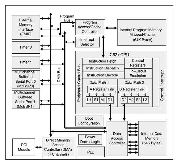
Figure 2. TMS320C6205 DSP Block Diagram
