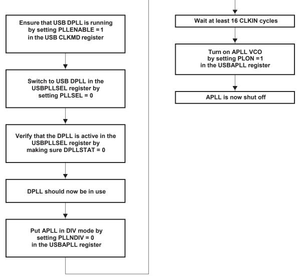
Figure 7. Switching to the DPLL From the APLL
