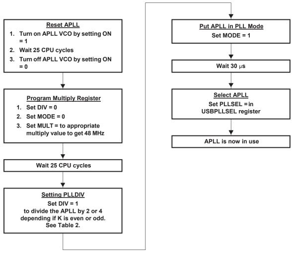
Figure 6. Switching to the APLL From the DPLL
