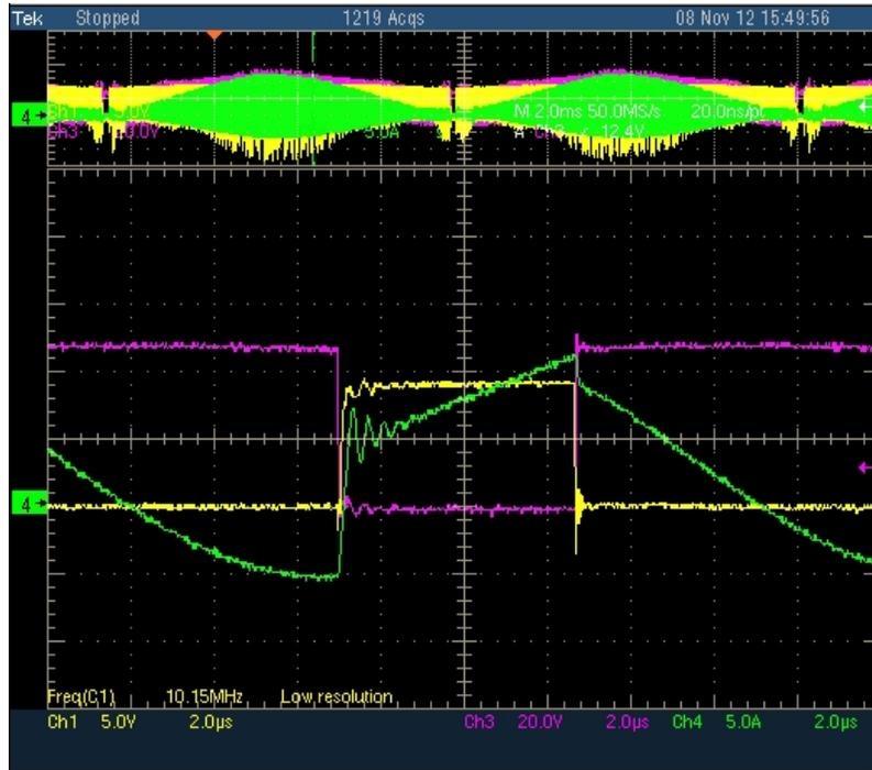
(CH1  $V_{GS}$  of main switch MOSFET,
