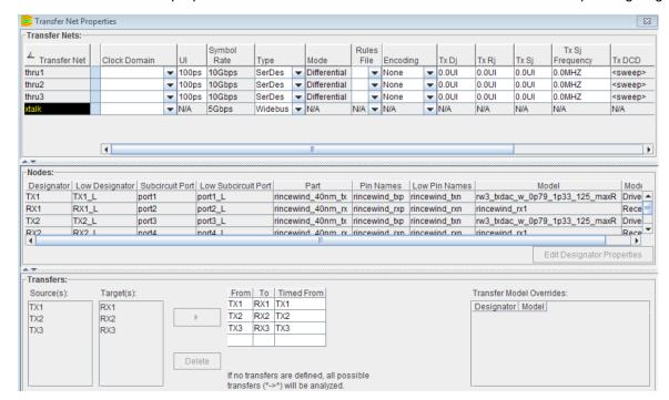
Figure 11. SiSoft QCD – Setting the Transfers in the Transfer Net Properties
