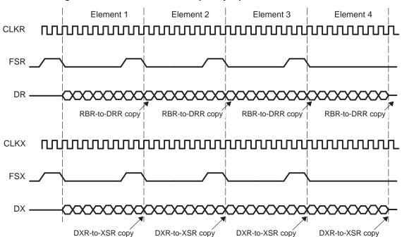
Figure 21. Maximum Frame Frequency Operation With 8-Bit Data
