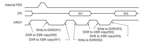
(d) XMCM = 3h, RPABLK = 0, XPABLK = x, RCERE0 = 0000 0008h, XCERE0 = 0000 000Ah: Receive channels: 1 and 3 enabled; transmit channels: 1 and 3 enabled, but only 3 unmasked
