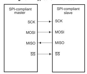
Figure 41. Typical SPI Interface
