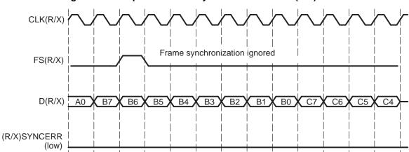
Figure 20. Unexpected Frame Synchronization With (R/X)FIG = 1
