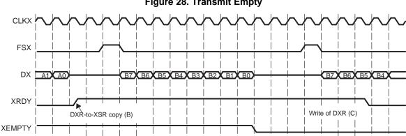
Figure 29. Transmit Empty Avoided **CLKX FSX** DX B6 X B5 X B4 X B3 X B2 X B1 C6 X C5 **XRDY** Write of DXR (C) DXR-to-XSR copy (B) DXR-to-XSR copy (C)
