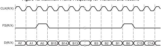
Figure 18. Maximum Frame Frequency for Transmit and Receive
