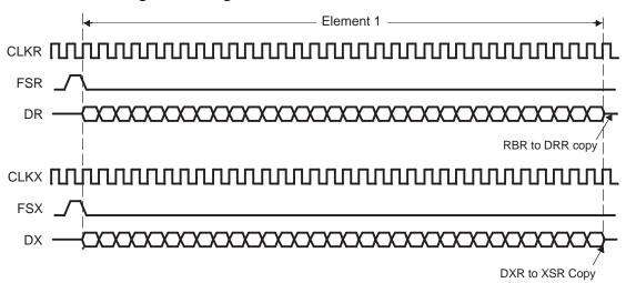
Figure 12. Single-Phase Frame of One 32-Bit Element
