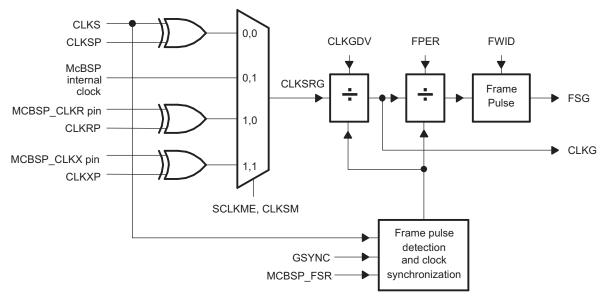
Figure 5. Sample Rate Generator Block Diagram
