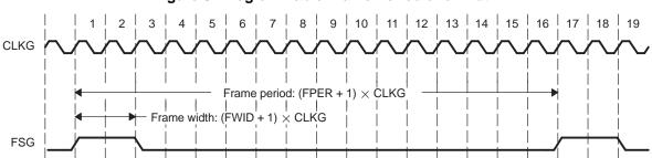
Figure 9. Programmable Frame Period and Width
