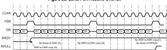
Figure 23. Serial Port Receive Overrun
