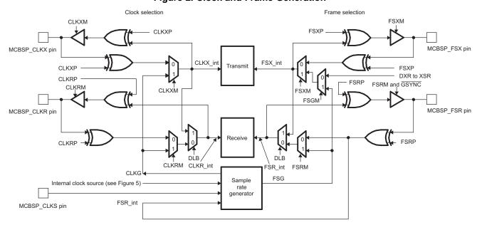
Figure 2. Clock and Frame Generation
