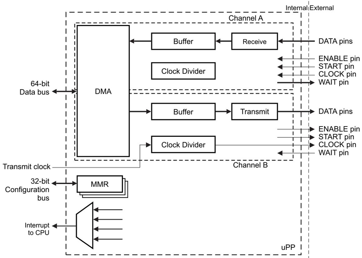
Figure 2. Data Flow for Single-Channel Receive Mode
