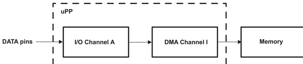
Figure 3. Data Flow for Single-Channel Transmit Mode
