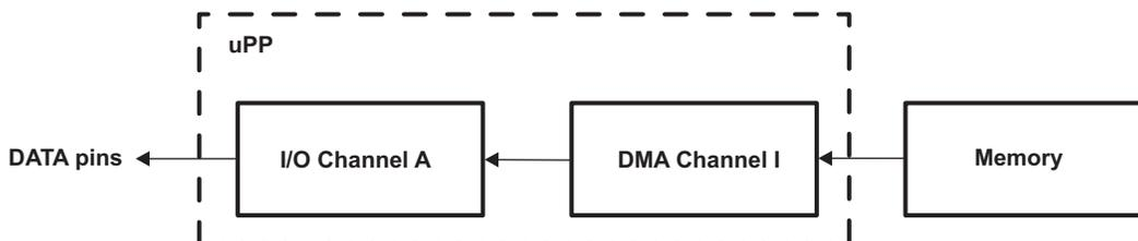
Figure 4. Data Flow for Digital Loopback (DLB) Mode (Duplex Mode 0)
