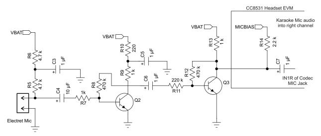
Figure 6. Karaoke MIC Audio into Right Channel
