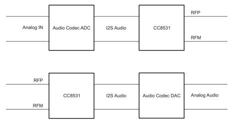
Figure 2. Audio Conversion Signal Chain
