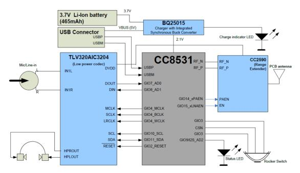
Figure 1. Typical CC85xx and TLV320AIC3204 Application Schematic
