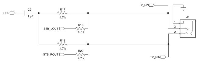
Figure 8. Add the Received Karaoke Sound to TV Audio Input
