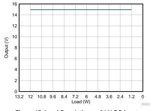
Figure 15. Load Regulation — 24-V DC Input
