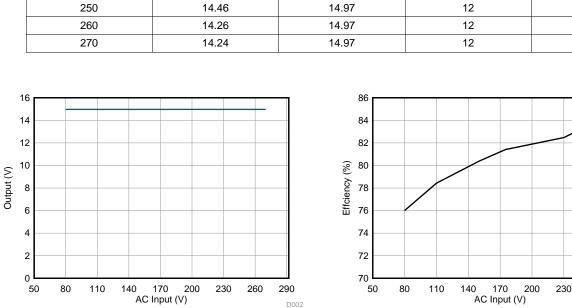
Figure 10. Output Voltage vs AC Input Voltage
