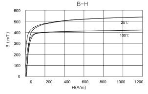
Figure 8. B-H Curve for Selected Core
