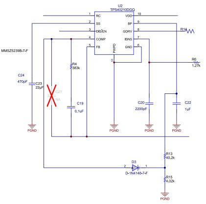
Figure 4. Duty Cycle Limiting Circuit
