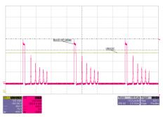
Figure 18. Booster Output  $V_{\mbox{\tiny BOOST}}$  and Booster FET Drain Voltage at 24-V DC Input
