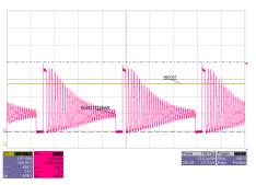
Figure 19. Booster Output  $V_{\mbox{\tiny BOOST}}$  and Booster FET Drain Voltage at 110-V DC Input
