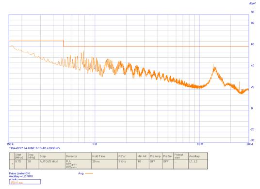
Figure 34. Test Result with Average-Mode Measurement — Tested at 230-V AC
