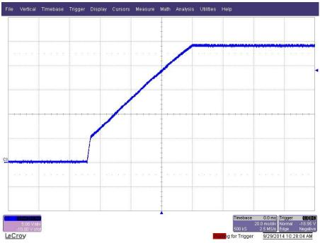
4.4 Start Up @ 400V<sub>AC</sub>: no load (200VAC/50Hz input with a voltage doubler circuit is applied here.).
