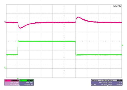
The photo below shows the 13.2V output voltage (ac coupled) when the load current is stepped between 1.5A and 3A. Vin = 12V. (500mV/DIV, 1A/DIV, 1mS/DIV)
