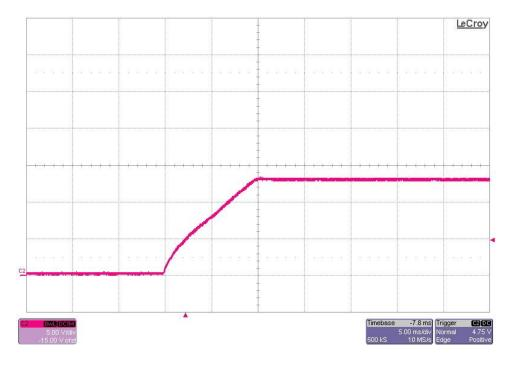
The photo below shows the output voltage startup waveform after the application of 6V in. The 13.2V output was loaded to 3A. (5V/DIV, 5mS/DIV)
