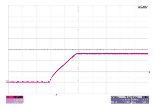
The photo below shows the output voltage startup waveform after the application of 16V in. The 13.2V output was loaded to 3A. (5V/DIV, 5mS/DIV)
