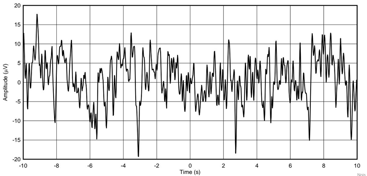
**Figure 13. Measured Output Noise at Full-Scale Code**
