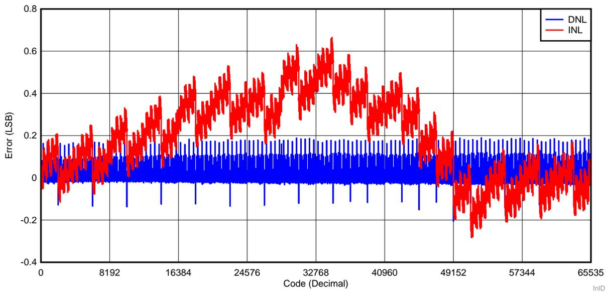
**Figure 12. Measured INL and DNL Errors**
