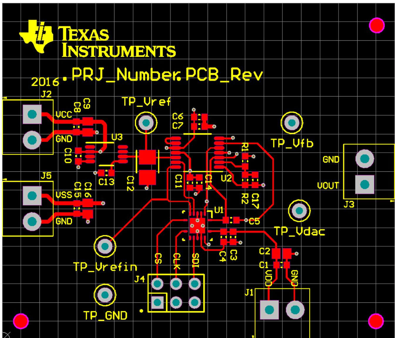
Figure 15. Top Side of PCB Layout
