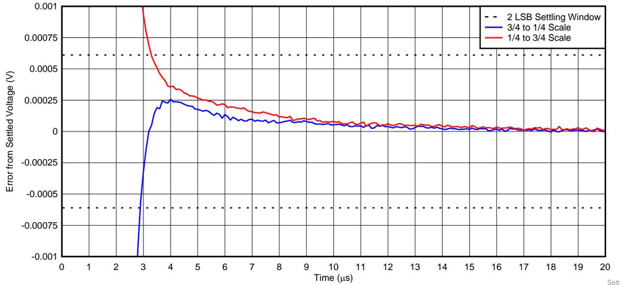
Figure 14. Measured Settling Time
