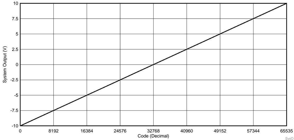
Figure 10. Measured System Transfer Function
