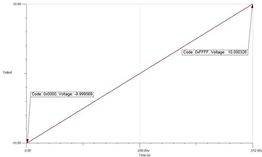
**Figure 8. TINA-TI™ Simulated Transfer Function**
