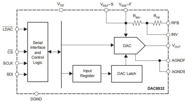
**Figure 6. DAC8832 Block Diagram**
