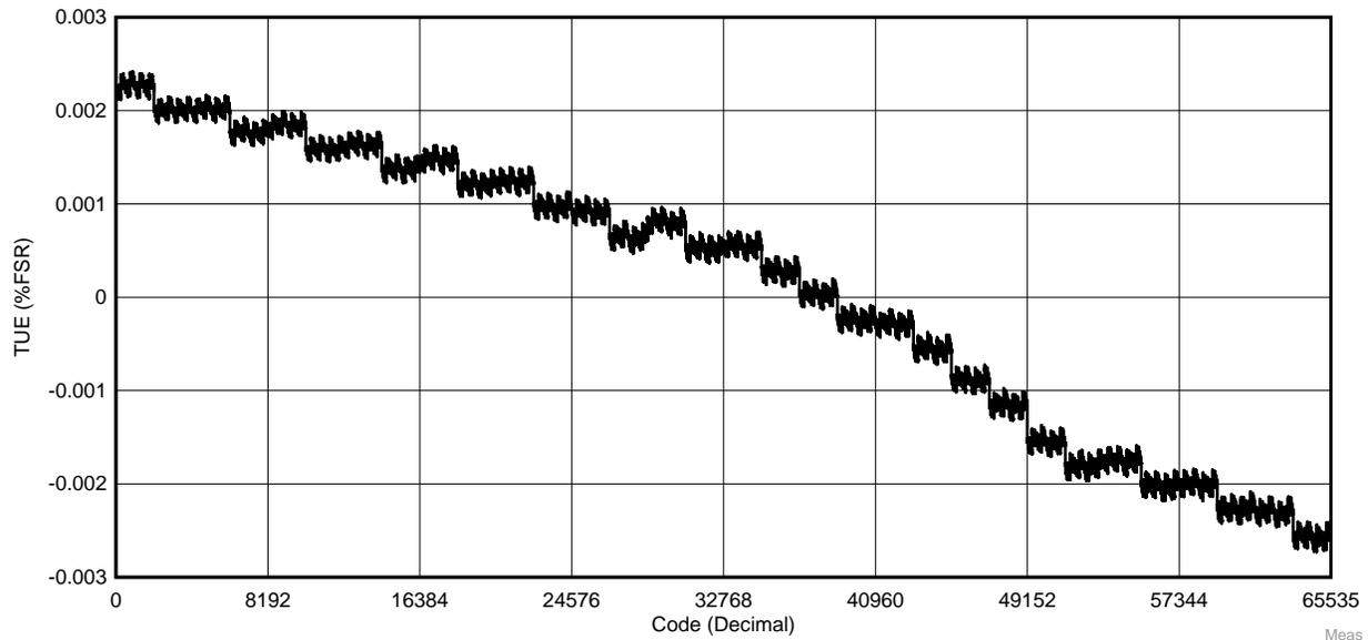
**Figure 1. Measured Total Unadjusted Error**
