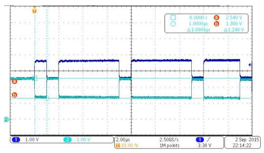
Figure 36. CANL Level During Transmit
