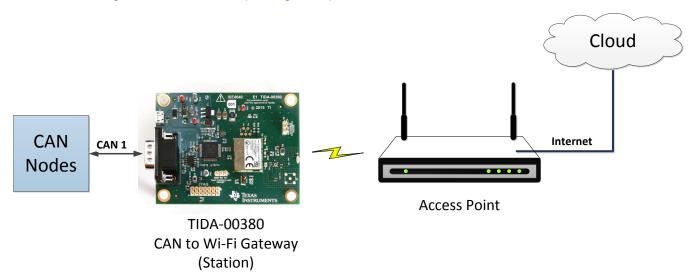
Figure 38. CAN-to-Wi-Fi® Gateway With Internet Cloud Interface
