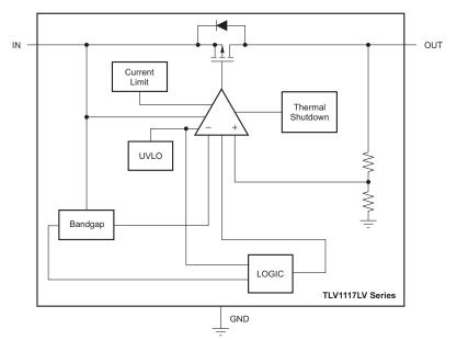
Figure 7. TLV1117LV33 Functional Block Diagram
