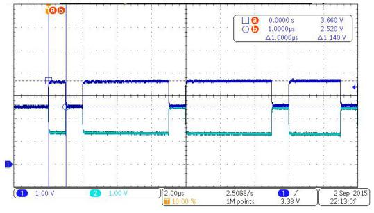
Figure 35. CAN SOF Timing Measurement Plus CANH Level During Transmit
