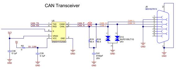
Figure 11. CAN Transceiver Schematic
