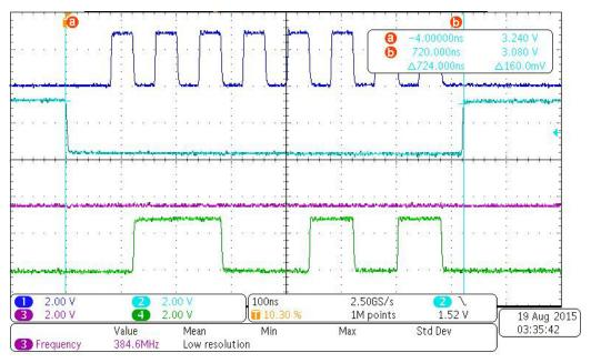
Figure 33. SPI Chip Select (CS) Period
