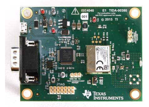
Figure 1. CAN to Wi-Fi® Gateway
