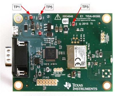
Figure 29. Locations of Test Points Used During Power Tests
