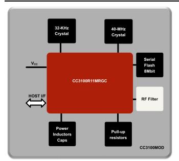
Figure 3. CC3100MOD Functional Block Diagram
