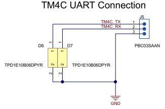
Figure 14. TM4C123GH6PM UART Terminal Connector Schematic
