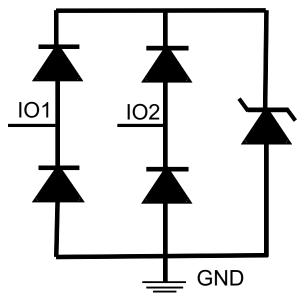
Figure 9. TPD2E2U06 Functional Block Diagram
