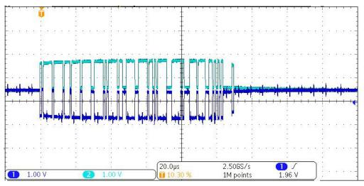
Figure 34. CAN Transmit from SN65HVD256
