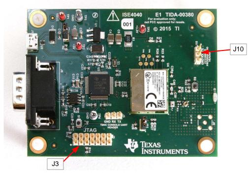
Figure 19. JTAG and UART Connections for Programming
