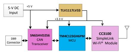
Figure 2. TIDA-00380 System Block Diagram
