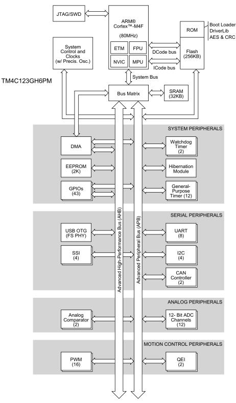
Figure 5. TM4C123GH6PM High-Level Block Diagram
