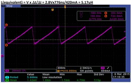
Figure 10. Inductor Current Ripple (2x8 LEDs), L = 4.7μH, TA = 85C, IOUT = 40mA
