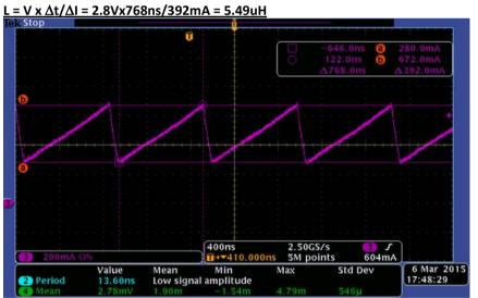
Figure 11. Inductor Current Ripple (2x8 LEDs), L = 4.7µH, TA = 25C, IOUT = 40mA
