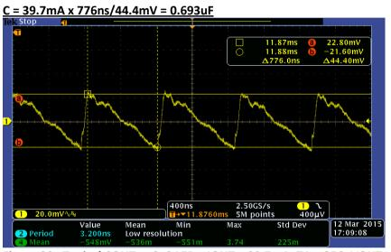
Figure 29. Typical COUT at 2x8 LEDs, IOUT = 39.7mA, TA = 25C, VOUT = 25.4V)
