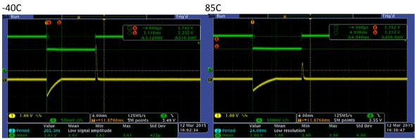
Figure 27. Line Voltage Steps (3.7V to 3.2V), L = 4.7uH, IOUT = 40mA
