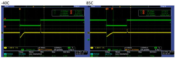
Figure 28. Line Voltage Steps (4.2V to 3.7V), L = 4.7uH, IOUT = 40mA
