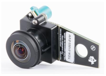
Figure 11. TIDA-01003 Completed Assembly
