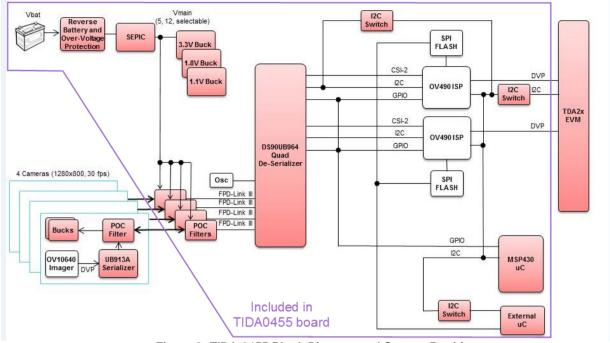
Figure 3: TIDA-0455 Block Diagram and System Partition
