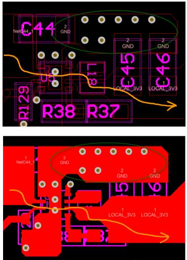
Figure 28: Step-Down Switch Mode Power Supply Routing
