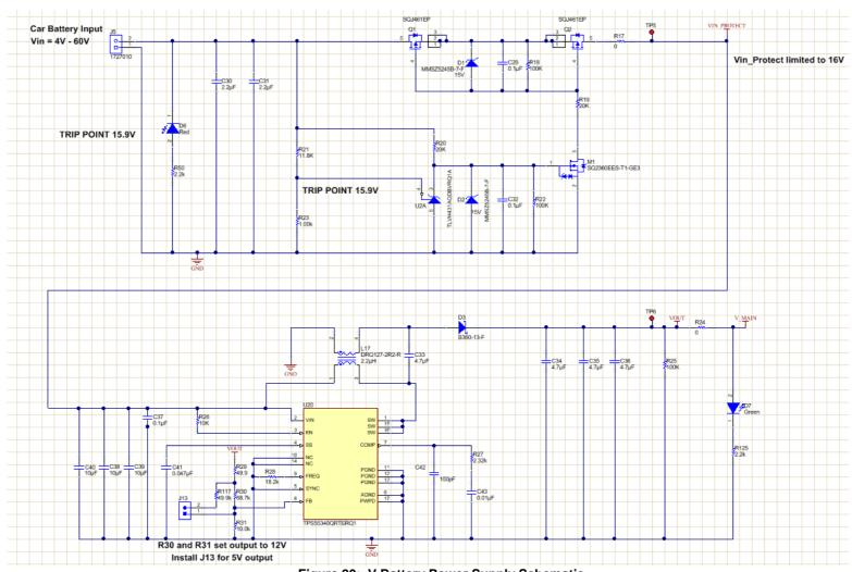
Figure 20: V Battery Power Supply Schematic
