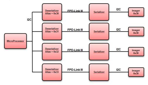
Figure 18: I2C Address Aliasing
