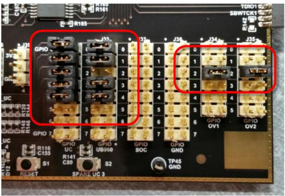
Figure 11: GPIO Jumpers
