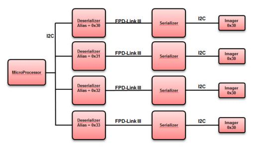
Figure 6: I2C Address Aliasing
