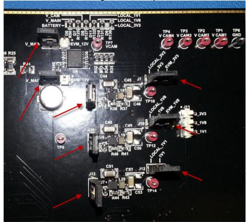
Figure 12: Power Supply Jumpers
