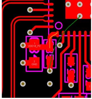
Figure 29: Decoupling Current Loop
