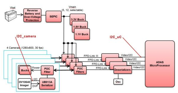
Figure 15: Setup for monitoring I2C transactions
