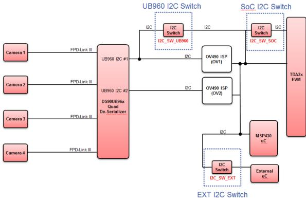
Figure 7: I2C Bus Diagram
