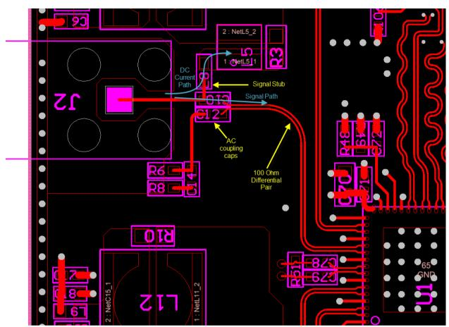
Figure 30: Decoupling Current Loop
