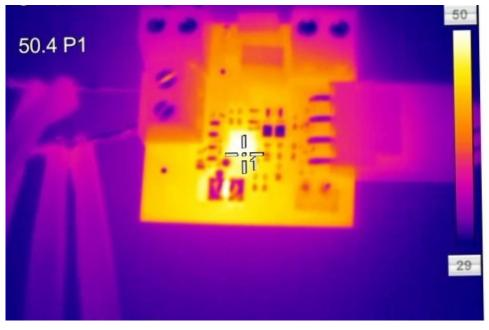
Figure 6. Thermal Performance at VBUS = 5 V and ICHG = 1.5 A
