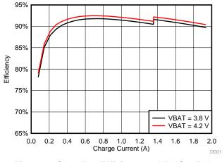
Figure 3. Charging Efficiency at VBUS = 5 V
