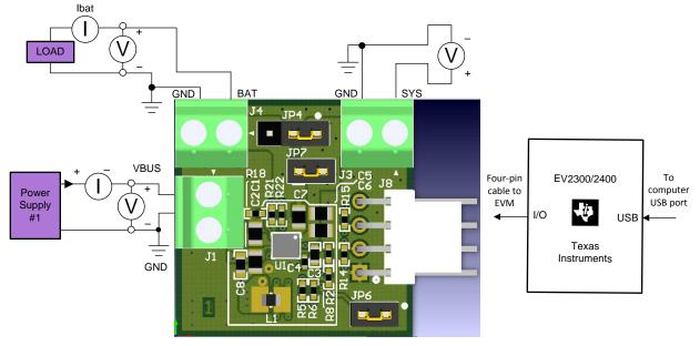
Figure 2. Test Setup
