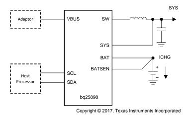
Figure 1. TIDA-03042 Block Diagram
