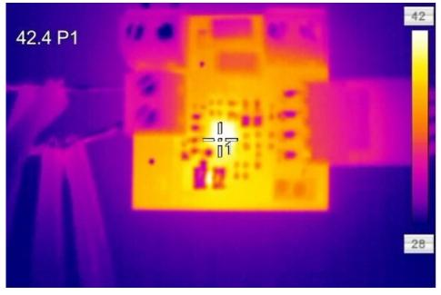
Figure 5. Thermal Performance at VBUS = 5 V and ICHG = 1 A
