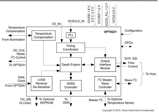
Figure 3. OPT9221 Functional Block Diagram
