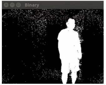
Figure 10. Background Subtraction Binary Image
