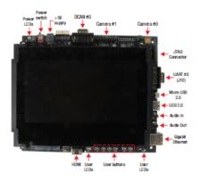
Figure 7. AM437x GP EVM Top View
