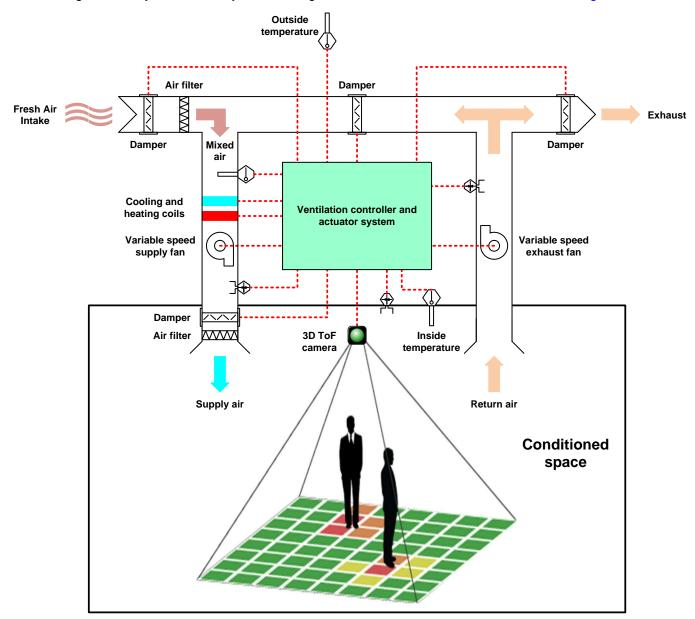
Figure 9. 3D ToF Camera Based DCV System
