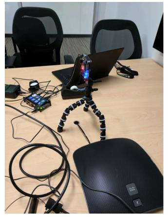
Figure 23. OPT8241 CDK and AM437x GP EVM With Tripod
