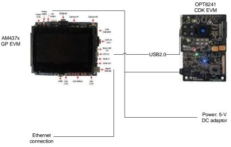
Figure 15. Hardware Setup
