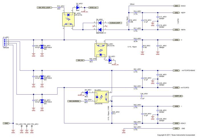
Figure 2. AFE Schematic of Channel With Conventional TVS Diodes
