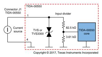
Figure 1. Block Diagram (One Channel)
