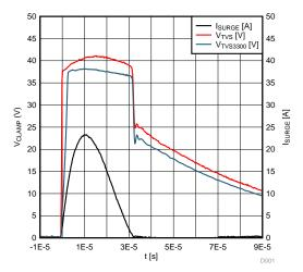
Figure 7. Clamping Voltage Over Surge Current
