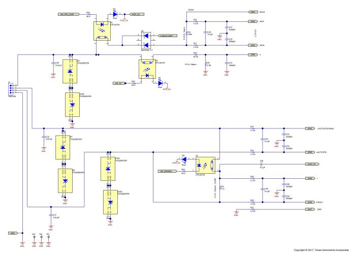
Figure 3. AFE Schematic of Channel With TVS3300
