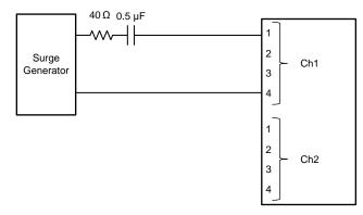
Figure 6. Surge Test Wiring Diagram
