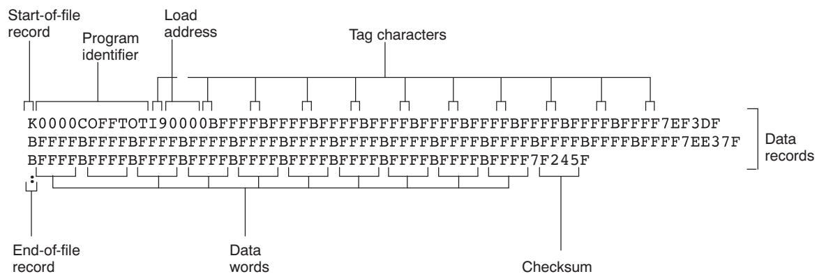
Figure 10-10. TI-Tagged Object Format
