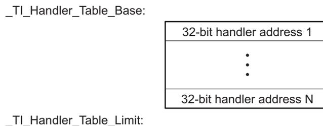
The linker creates a separate output section for the load and run space. For example, if .task1.load is compressed using RLE, the handler index points to an entry in the handler table that has the address of the run-time-support routine \_\_TI\_decompress\_rle().
