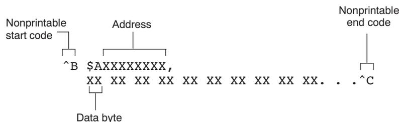
The file begins with an ASCII STX character (ctrl-B, 02h) and ends with an ASCII ETX character (ctrl-C, 03h). Address records are indicated with \$XXXXXXXX, in which XXXXXXXX is a 8-digit (16-bit) hexadecimal address. The address records are present only in the following situations:
