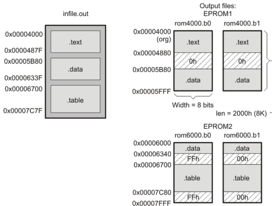
The map file (specified with the `--map` option) is advantageous when you use the ROMS directive with multiple ranges. The map file shows each range, its parameters, names of associated output files, and a list of contents (section names and fill values) broken down by address. [Example 10-2](#) is a segment of the map file resulting from the example in [Example 10-1](#).
