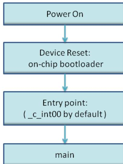
The primary bootloader is typically very small and copies a limited amount of memory from a dedicated location in ROM to a dedicated location in RAM. (Some bootloaders support copying the program from an I/O peripheral.) After the copy is completed, it transfers control to the program.
