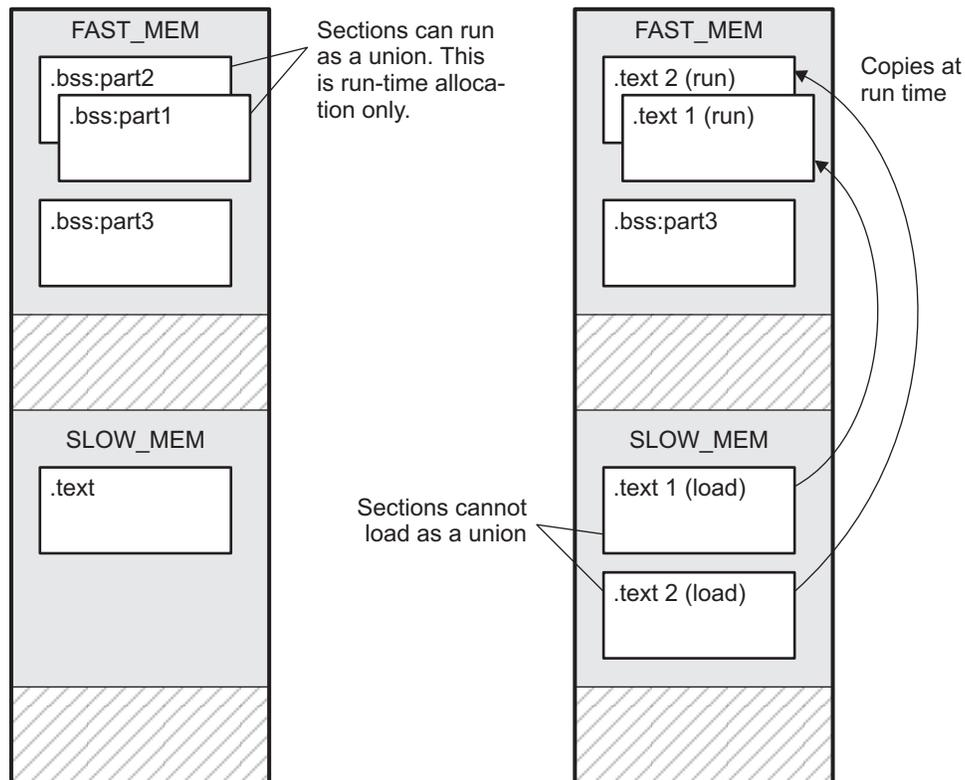
Since the .text sections contain raw data, they cannot *load* as a union, although they can be *run* as a union. Therefore, each requires its own load address. If you fail to provide a load allocation for an initialized section within a UNION, the linker issues a warning and allocates load space anywhere it can in configured memory.
