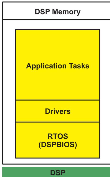
In this scenario, the DSP application is a single static executable file that contains: the RTOS, any required driver functions, and all tasks that the application needs to carry out. All of the addresses in the static executable are bound at link-time, they cannot be relocated at load-time. Execution of the DSP application will proceed from the application's entry point.
