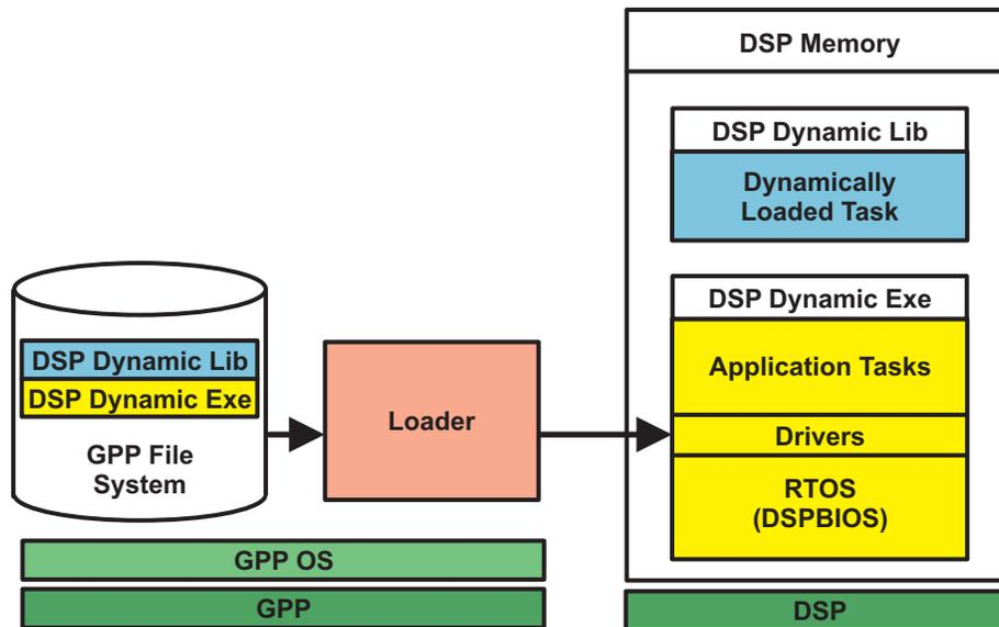
If we convert the earlier RTOS example into a dynamic system, the RTOS part of the system is still built like an executable and is assumed to be loaded by traditional means (bootstrap loader) and set running on the DSP by a host application.
