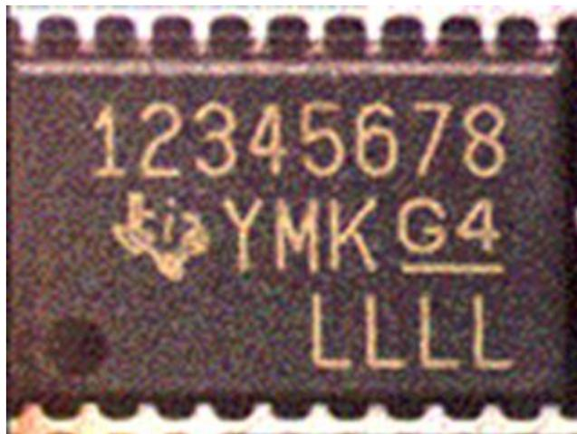
Example of Pb-free category marking on a 20-pin TSSOP package. 'G4' indicates NiPdAu finish on the component and use of "green" mold compound.
