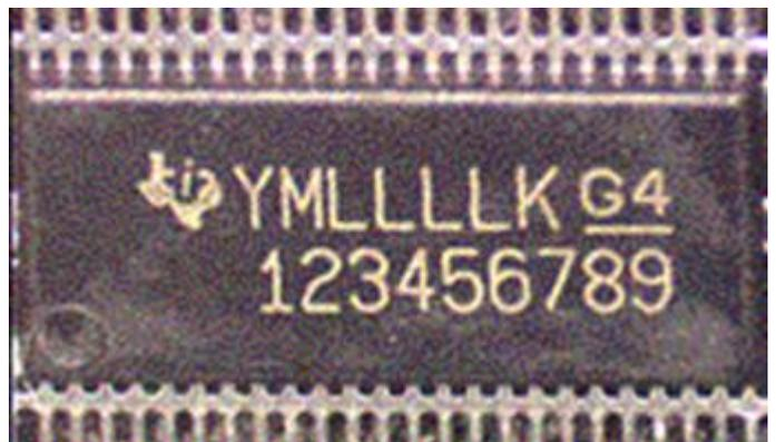
Example of Pb-free category symbolized on TI 56-pin TVSOP package. ‘G4’ indicates NiPdAu finish on the component with use of “green” mold compound.
