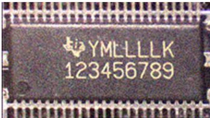
Example of a conventional marking format (no Pb Free designation) on a 56-pin TVSOP package.
