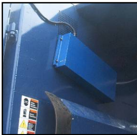
Truck-mounted RFID antenna
