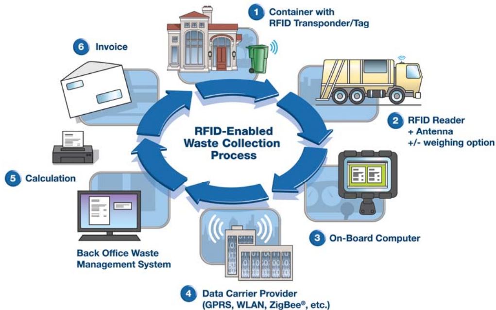
Figure 2 RFID and Technology Enabled Waste Management Cycle (Automation of the waste collection process)
