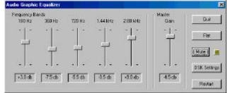
The five-band graphic equalizer uses five parallel 128<sup>th</sup> order FIR filters, with the gain of each filter independently controlled by a slider control. A master gain control, mute button, and flat button provide additional control.
