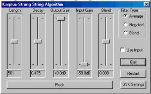
Implements the Karplus-Strong string algorithm [2] to synthesize a plucked string. The delay buffer length, decay coefficient, and the filter type are all user adjustable. Additionally, the ADC input can be processed through the algorithm by using it to excite the string buffer on a continuous basis.
