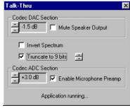
This application takes audio input from the ADC and passes it back out through the DAC. All aspects of the TLC320AD535 CODEC on the DSK can be controlled. The user can also vary the effective number of bits from the full 15-bit range of the AIC down to a single bit, demonstrating the relationship between quantization and signal-to-noise ratio. The concept of spectral inversion can also be demonstrated.
