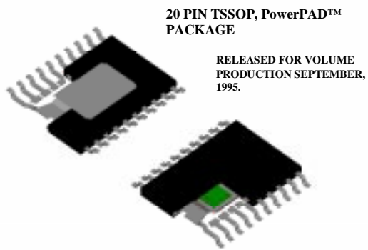
Figure 8. Top and Bottom section view of the 20 pin TSSOP PowerPAD™ package that was first introduced in 1995. This version has the 4 corner package leads tied to the die pad for enhanced thermal efficiency (a standard option in PowerPAD™ packages), in addition to the die pad exposed at the surface of the package body.
