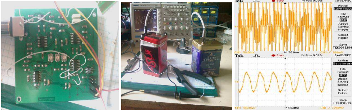
Picture 9. Amplifier board, generator connected with amplifier and signal before and after amplification with filtration
