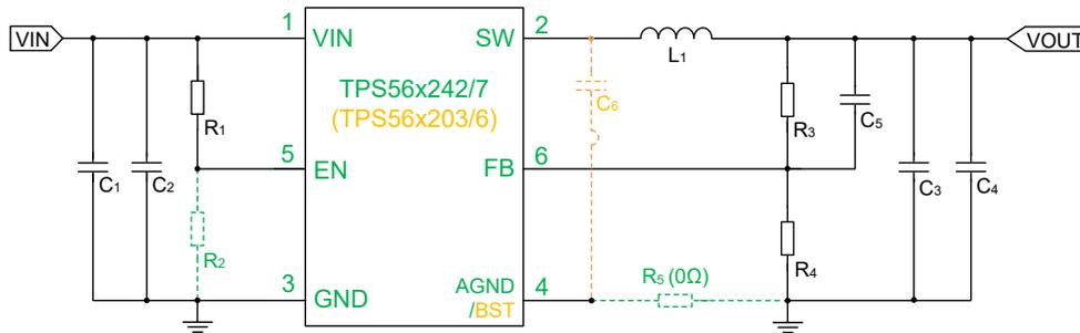
**Figure 3-4. Co-Layout Schematic for TPS56x242/7 and TPS56x203/6**
