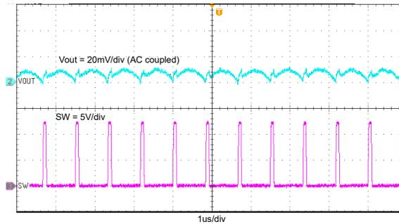
**Figure 4-3. TPS563252 12V Input to 1.05V Output at 3A**
