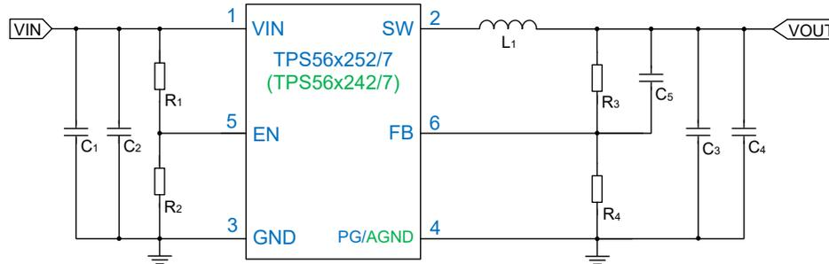
Figure 3-2. Co-Layout Schematic for TPS56x252/7 and TPS56x242/7
