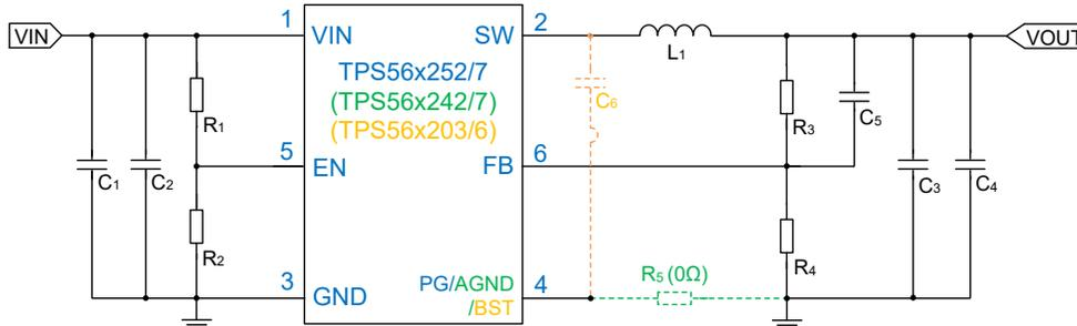
Figure 3-1. Co-layout Schematic Among Three Types of SOT-563
