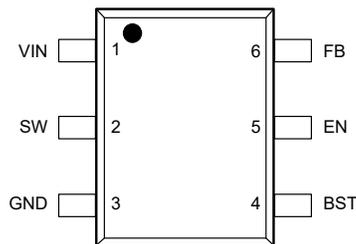
Figure 2-1. TPS56x203/6 Pinout
