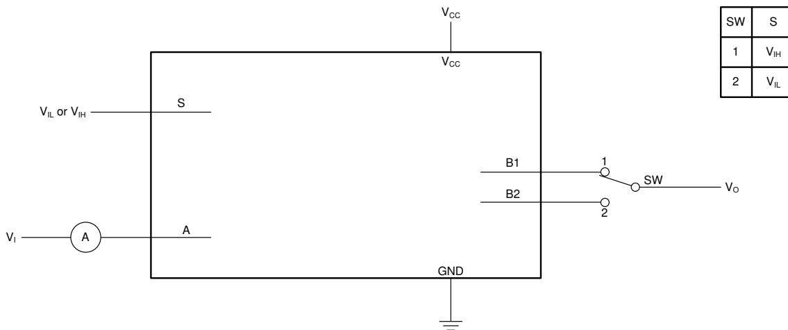
图 7-2. OFF-State Switch Leakage-Current Test Circuit
