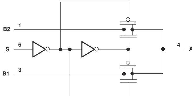
図 8-1. Logic Diagram (Positive Logic)
