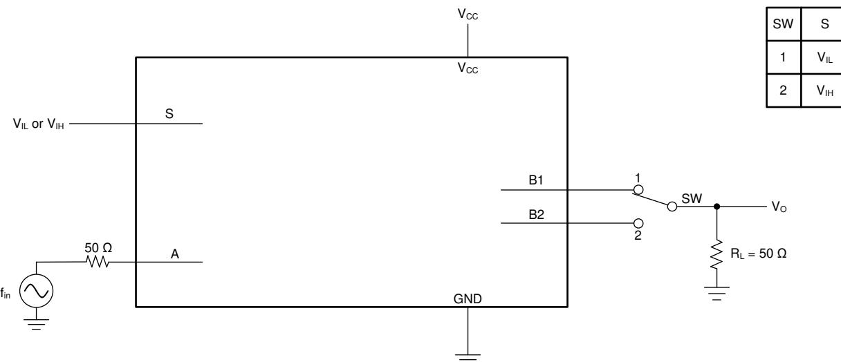
図 7-5. Frequency Response (Switch On)
