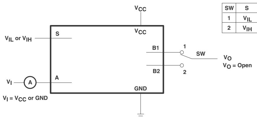
图 7-3. ON-State Switch Leakage-Current Test Circuit
