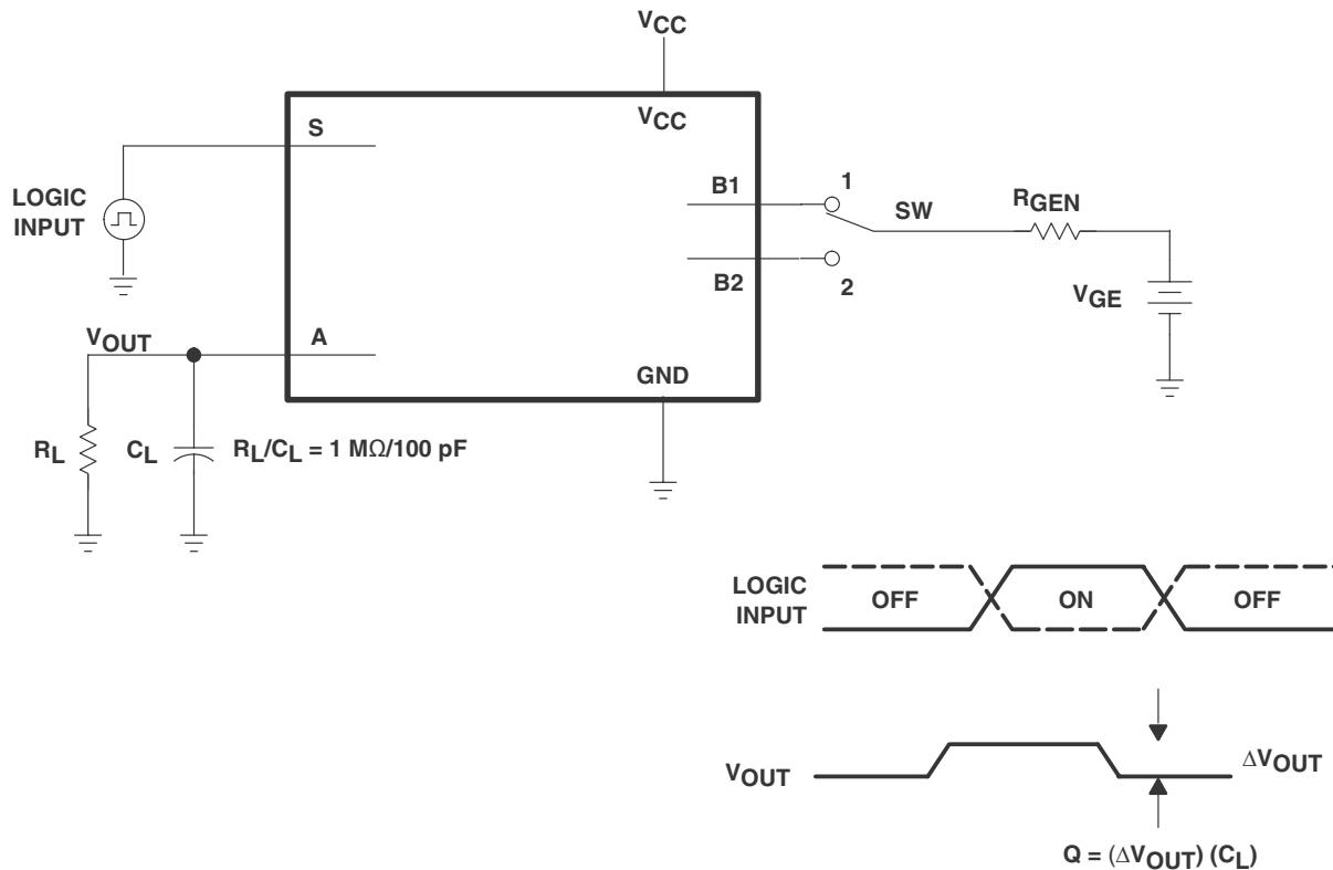
図 7-8. Charge-Injection Test
