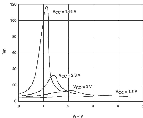
図 6-1. Typical  $r_{on}$  as a Function of Input Voltage ( $V_I$ ) for  $V_I = 0$  to  $V_{CC}$
