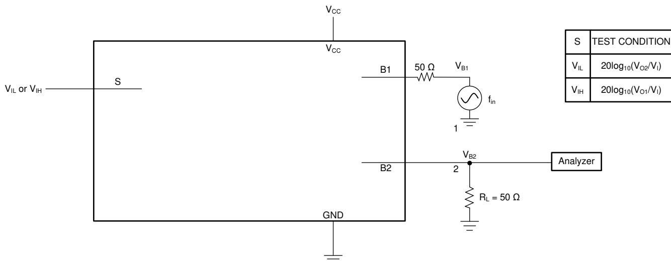
図 7-6. Crosstalk (Between Switches)
