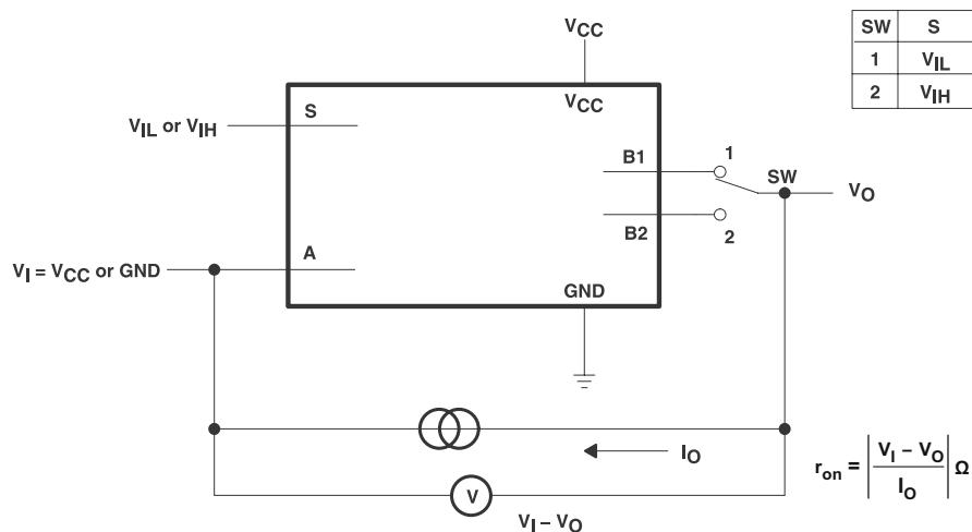
图 7-1. ON-State Resistance Test Circuit
