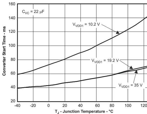
7-3. Converter Start Time vs Temperature
