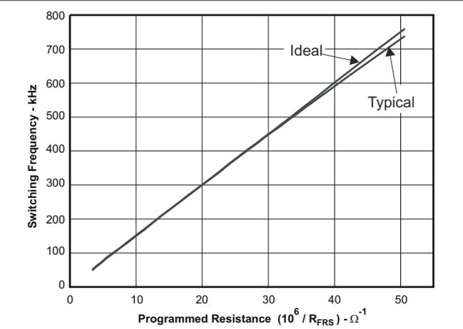
7-8. Switching Frequency vs Programmed Resistance
