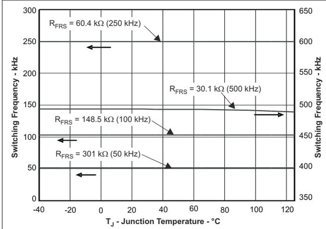
7-7. Switching Frequency vs Temperature
