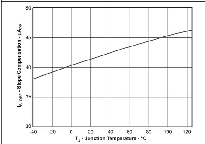
7-11. Current Slope Compensation Current vs Temperature
