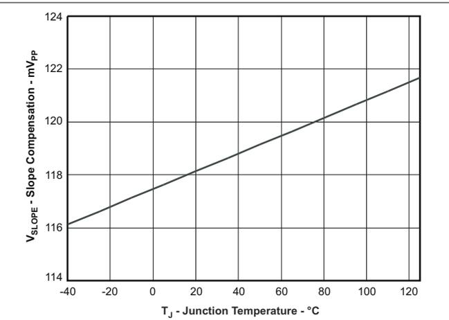
7-10. Current Slope Compensation Voltage vs Temperature
