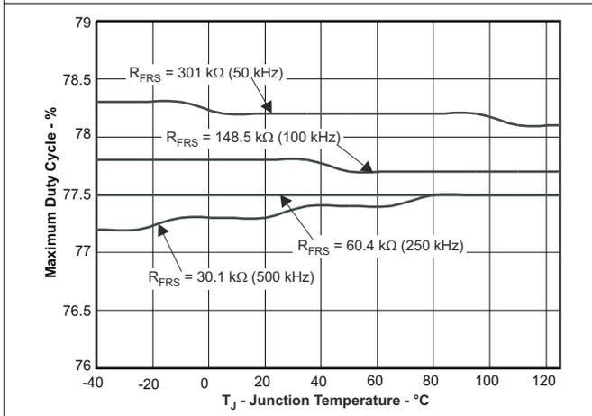
7-9. Maximum Duty Cycle vs Temperature
