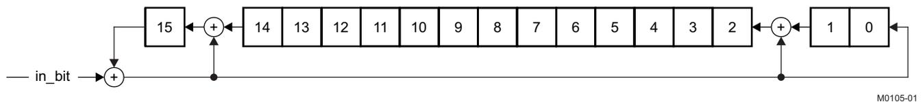
Figure 14-1. Basic Structure of the Random-Number Generator
