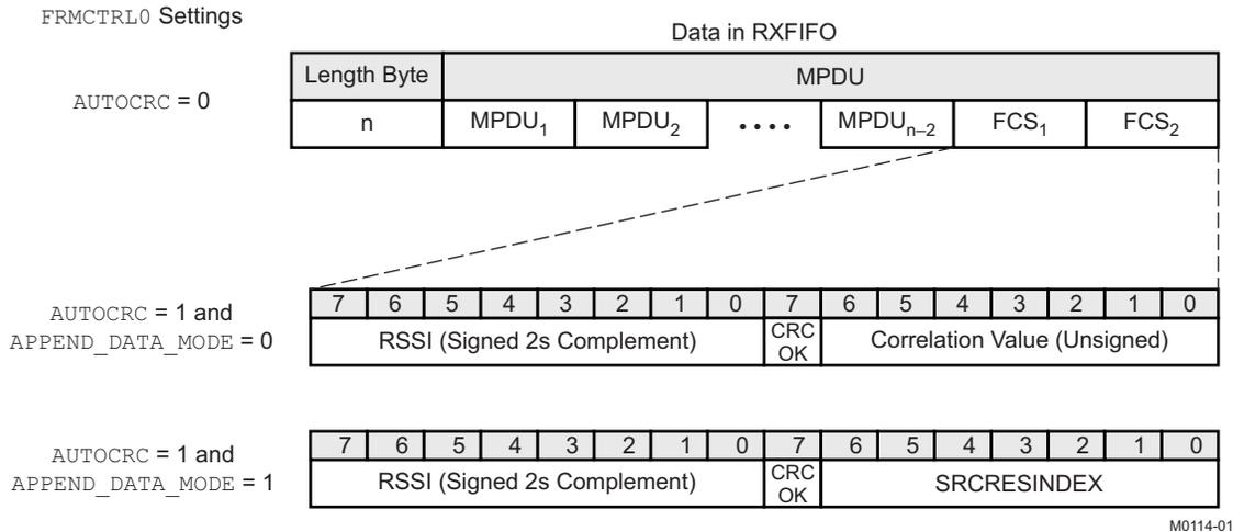
**Figure 23-15. Data in RXFIFO for Different Settings**
