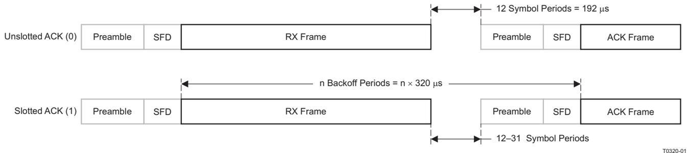
Figure 23-17. Acknowledgment Timing
