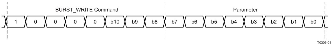
Figure 3-5. Burst Write Command (First 2 Bytes)
