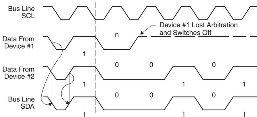
Figure 20-7. Arbitration Procedure Between Two Master Transmitters
