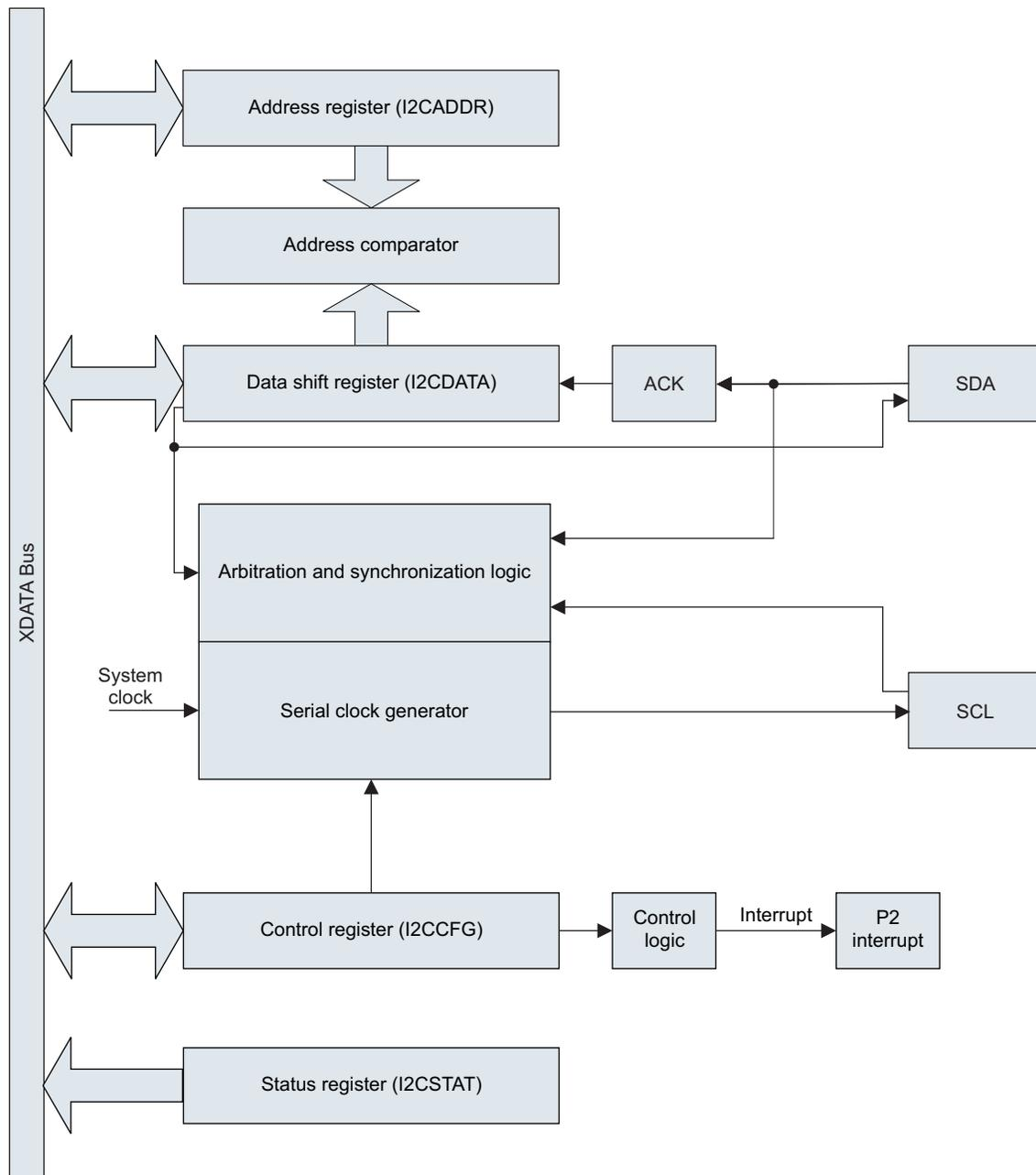
Figure 20-1. Block Diagram of the I<sup>2</sup>C Module
