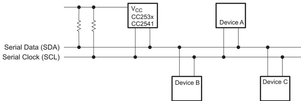
**Figure 20-2. I<sup>2</sup>C Bus Connection Diagram**
