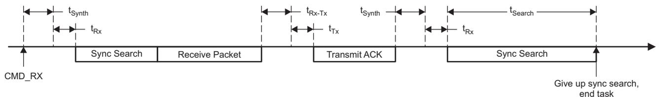
NOTE: The time given by  $PRF\_SEARCH\_TIME$  is denoted  $t_{Search}$  and the time given by  $PRF\_RX\_TX$  is denoted  $t_{Rx-Tx}$ . The setup and wait time for the synthesizer, receiver, and transmitter are denoted  $t_{Synth}$ ,  $t_{Tx}$ , and  $t_{Rx}$ , respectively.
