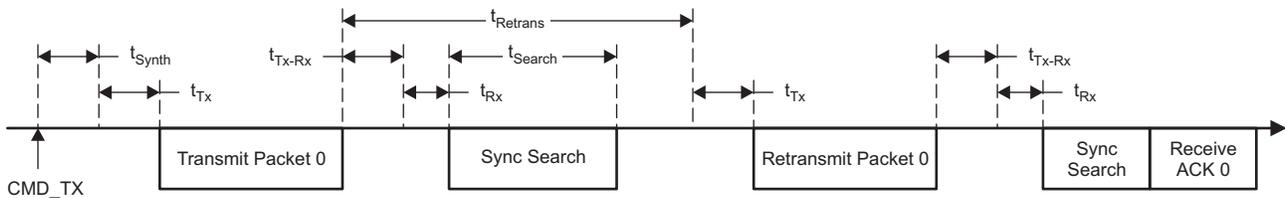
Transmit task, `PRF_TASK_CONF.MODE = 1X`, `.START_CONF = 0`, `.REPEAT = 1`, CRC error on ACK:
