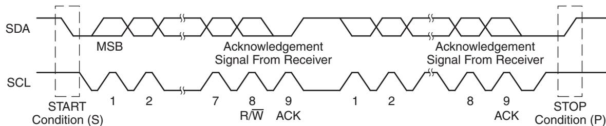
**Figure 20-3. I<sup>2</sup>C Module Data Transfer**
