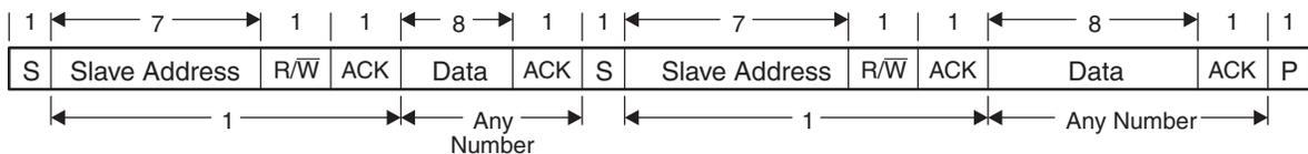
Figure 20-6. I<sup>2</sup>C Module Addressing Format With Repeated START Condition
