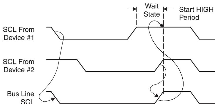
Figure 20-8. Synchronization of Two I<sup>2</sup>C Clock Generators During Arbitration
