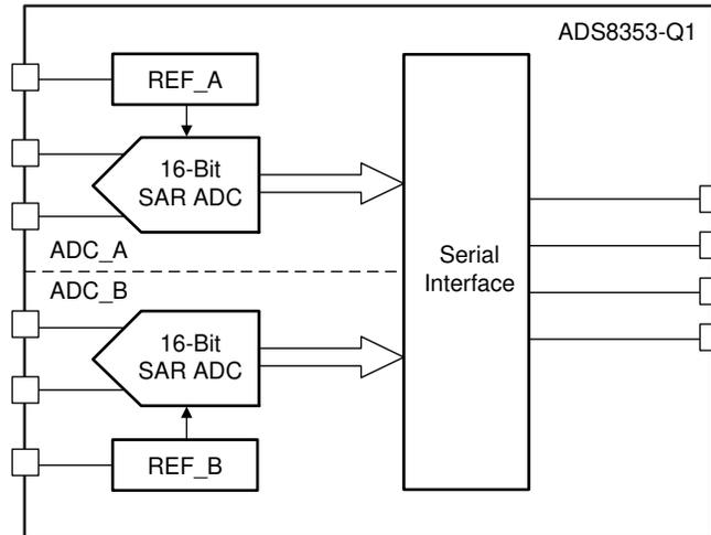
**Figure 1-1. Functional Block Diagram**
