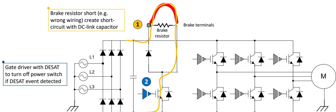
Figure 1-2. Short Circuit Due to Miswiring of External Brake Resistor Terminal
