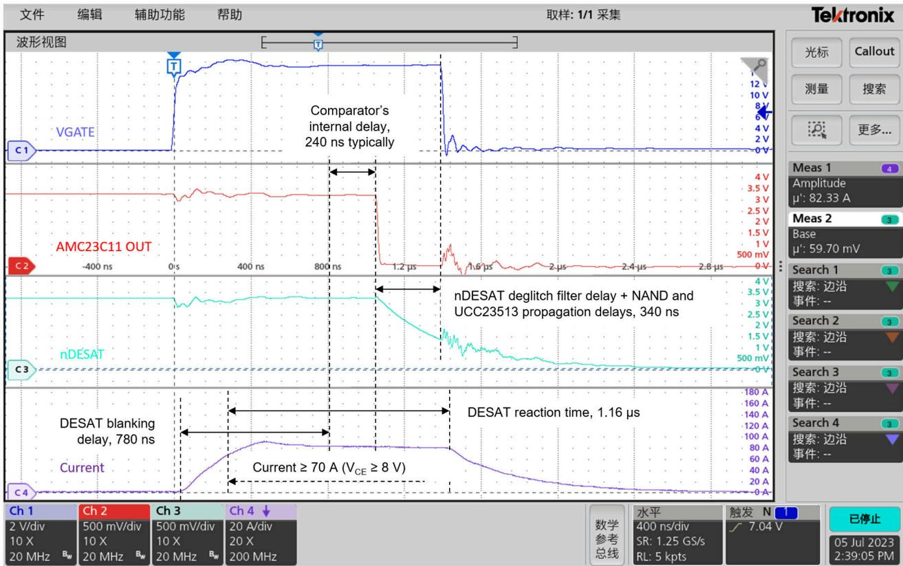
Figure 4-4. Short-Circuit Protection Delays in Low-side Driving Test
