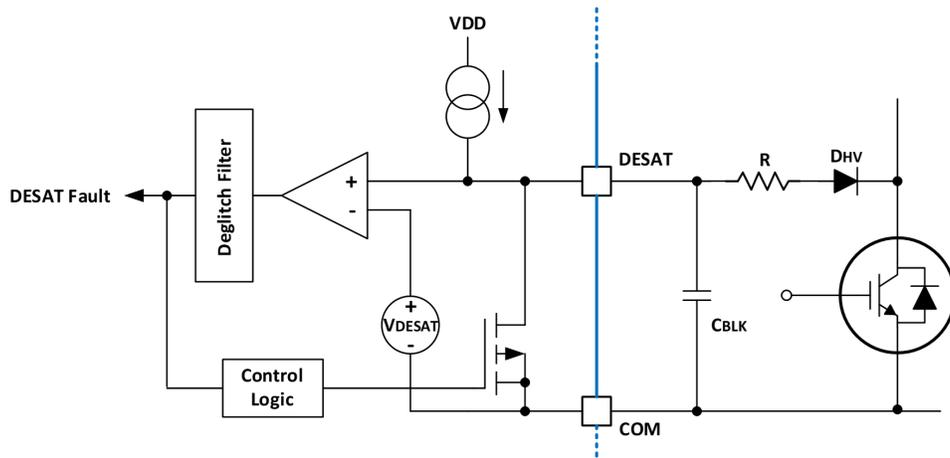
**Figure 1-3. UCC21750 With Integrated DESAT Protection**
