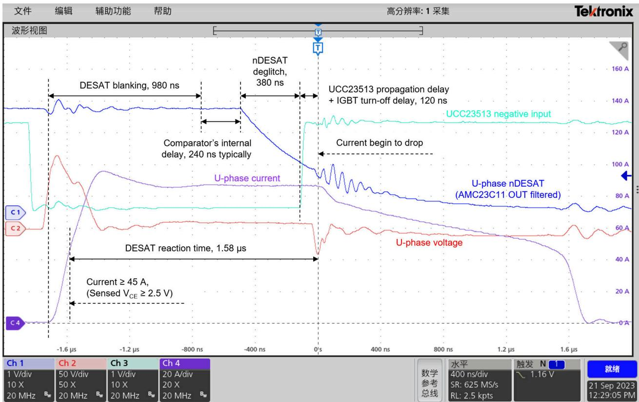
Figure 4-6. Short-Circuit Protection Delays in Run Motor Test
