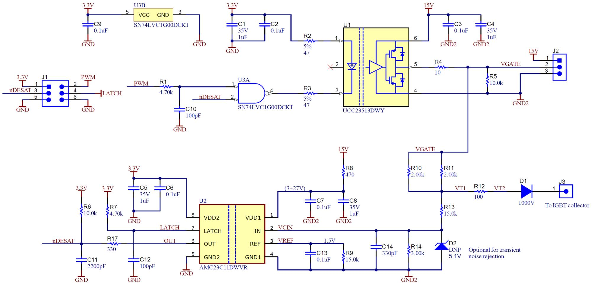
Figure 3-2. Schematic of the Proposed Circuit
