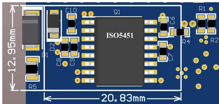
**Figure 3-4. Typical Layout of the Smart Gate Driver ISO5451**
