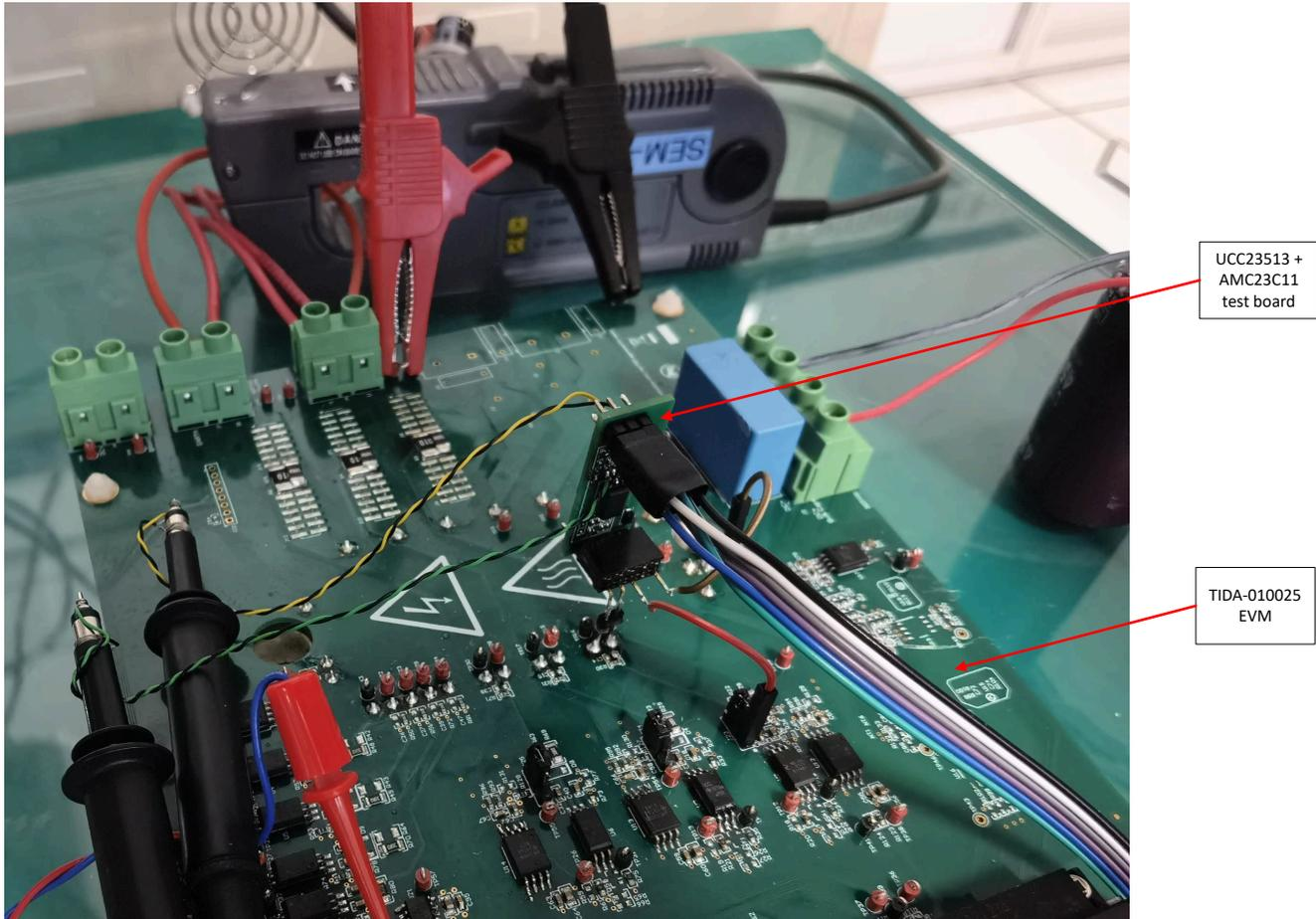
**Figure 4-5. Platform for Run Motor Test**
