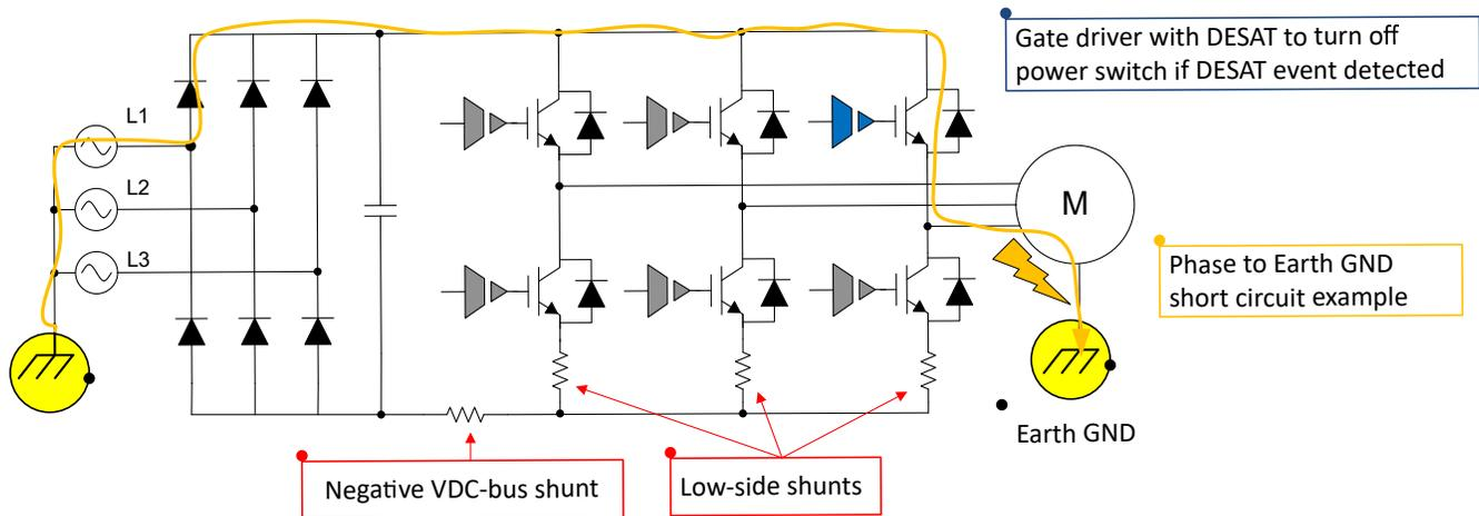
Figure 1-1. Short Circuit Due to Earth Ground Fault in A 3-Phase Inverter
