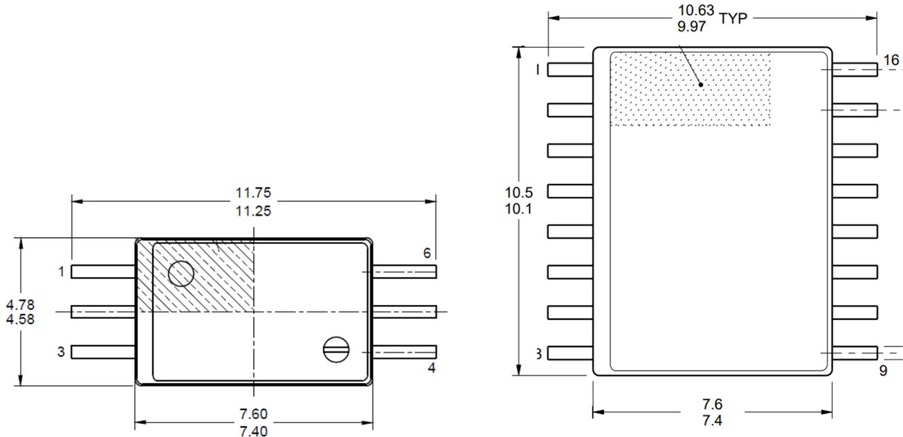
**Figure 2-1. Package Size Comparison: SO-6 vs. SOIC-16**
