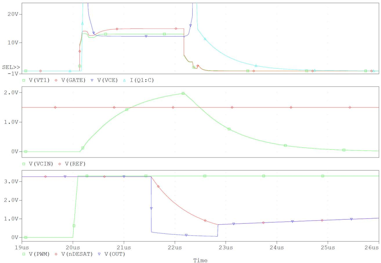
**Figure 4-2. Simulation Result of DESAT Triggered**
