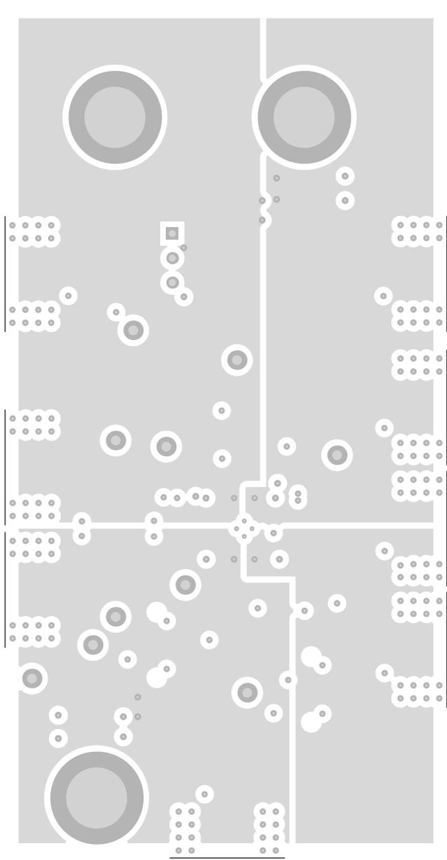
Figure 10. Layer 3: Power Plane,  $\pm V_{cc}$
