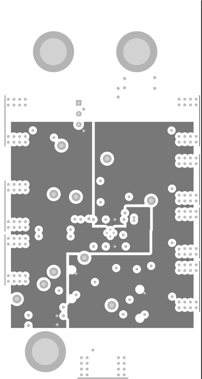
Figure 11. Layer 4: Power Plane,  $\pm V_{cc}$
