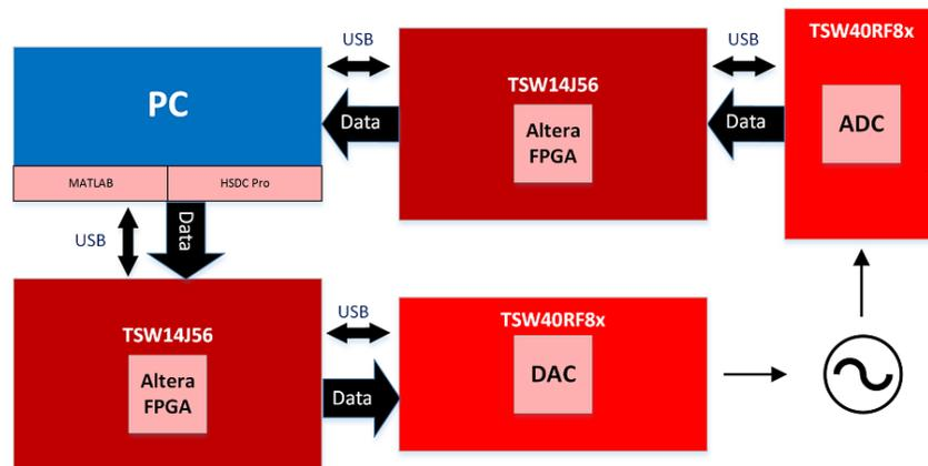
**Figure 1. Block Diagram of Setup**
