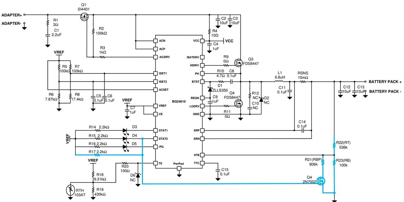
$V_{\text{IN}} = 18 \text{ V to } 28 \text{ V}$ ,  $V_{\text{topping}} = 14.7 \text{ V}$ ,  $I_{\text{charge}} = 2.4 \text{ A}$ ,  $I_{\text{pre-charge}} = I_{\text{term}} = 0.24 \text{ A}$ , 10-hour safety timer
