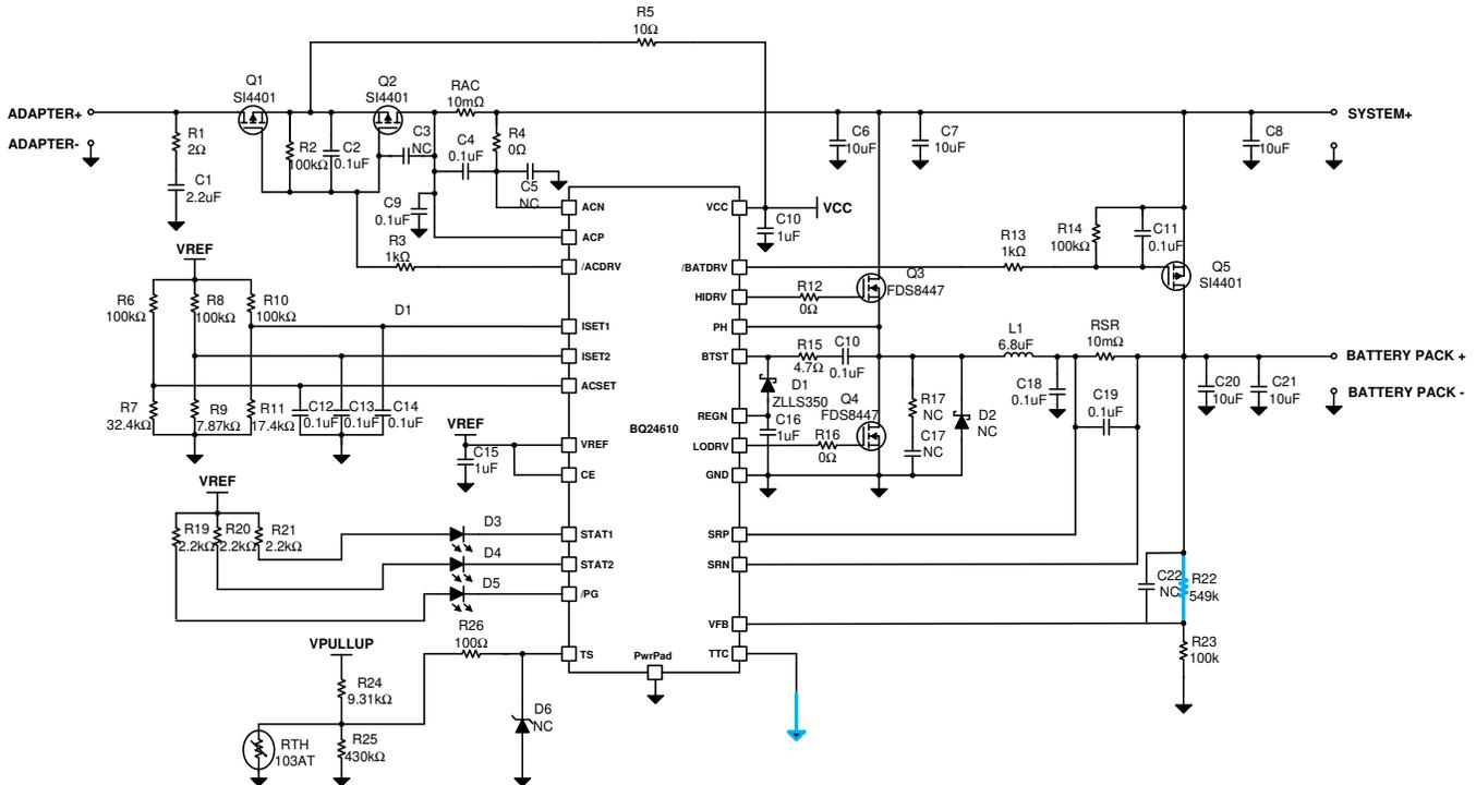
$V_{IN} = 18\text{ V to }28\text{ V}$ ,  $V_{float} = 13.7\text{ V}$ ,  $I_{charge} = 2.4\text{ A}$ ,  $I_{pre-charge} = 0.24\text{ A}$ , with power path selector
