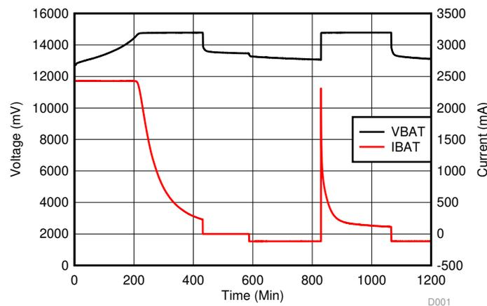
**Figure 5. Measured Charging Profile for Repeating Applications**
