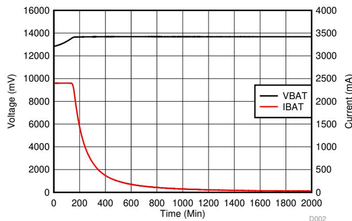
**Figure 6. Measured Charging Profile for Backup Applications**
