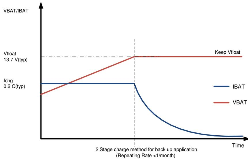
**Figure 3. Charging Profile for Backup Applications**
