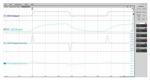
Figure 4-4. Transient Switching Current for SN74AVCxT245 and SN74LXCxT245
