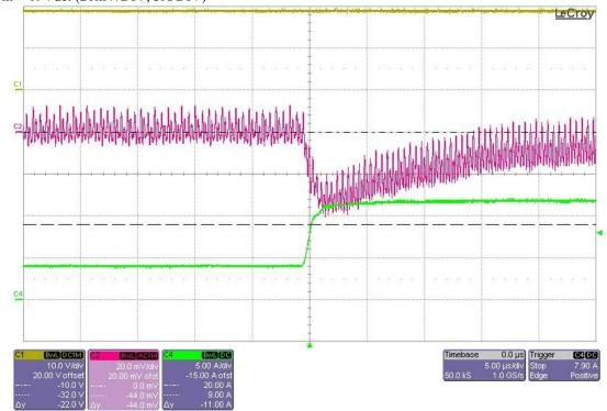
The photo below shows the output voltage deviation of 44mV ( $\sim 4\%\text{Vout}$ ) when the load current is pulsed from 0A to 6A. Vin = 19Vdc. (20mV/DIV, 5A/DIV)
