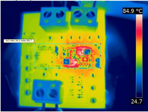
The converter temperature profile is shown below at Vin = 19V, Iout= 8A.
