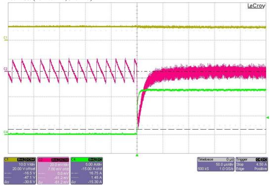
The photo below shows the output voltage when the load current is pulsed from 4A to 12A. Vin = 7.2Vdc. (20mV/DIV, 5A/DIV)
