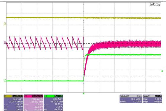
The photo below shows the output voltage when the load current is pulsed from 4A to 12A. Vin = 6Vdc. (20mV/DIV, 5A/DIV)
