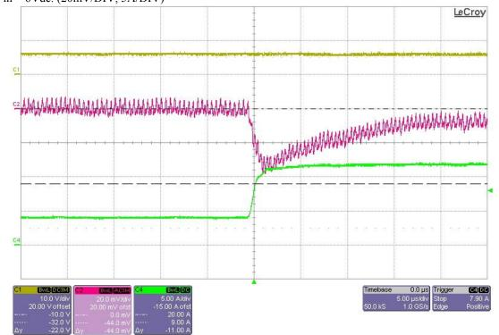
The photo below shows the output voltage deviation of 44mV (~4%Vout) when the load current is pulsed from 0A to 7.5A. Vin = 6Vdc. (20mV/DIV, 5A/DIV)
