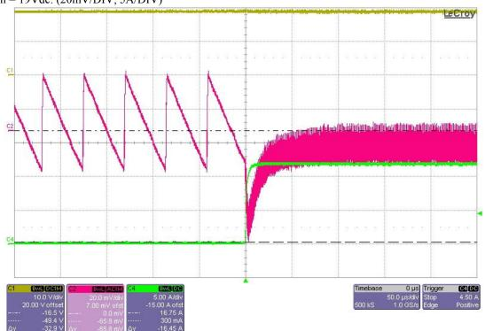
The photo below shows the output voltage when the load current is pulsed from 4A to 12A. Vin = 19Vdc. (20mV/DIV, 5A/DIV)
