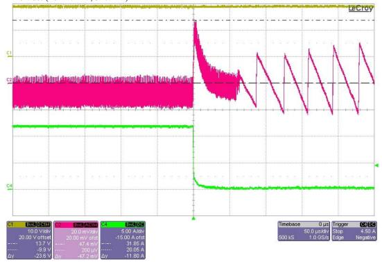
The photo below shows the output voltage when the load current is pulsed from 12A to 4A.
