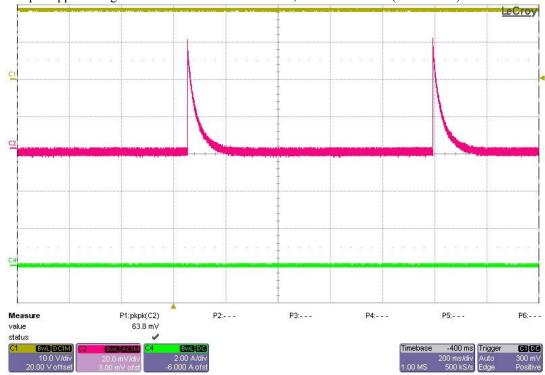
The output ripple voltage is shown in the figure below with Vin=19V, Iout = 100mA. (20mV/DIV)
