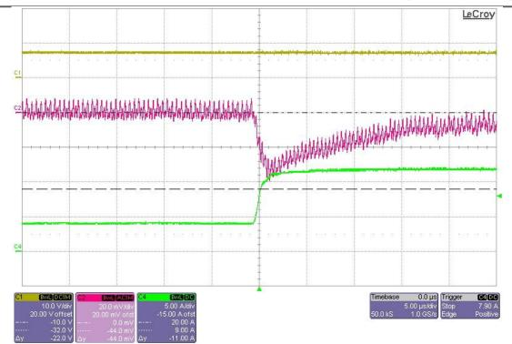
The photo below shows the output voltage deviation of 44mV ( $\sim 4\%\text{Vout}$ ) when the load current is pulsed from 0A to 7.5A. Vin = 7.2Vdc. (20mV/DIV, 5A/DIV)
