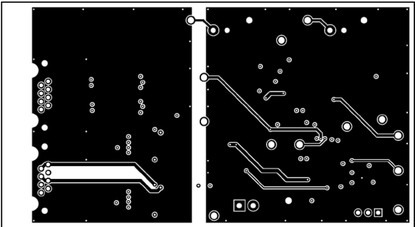
Figure 9. Layer 3 Routing
