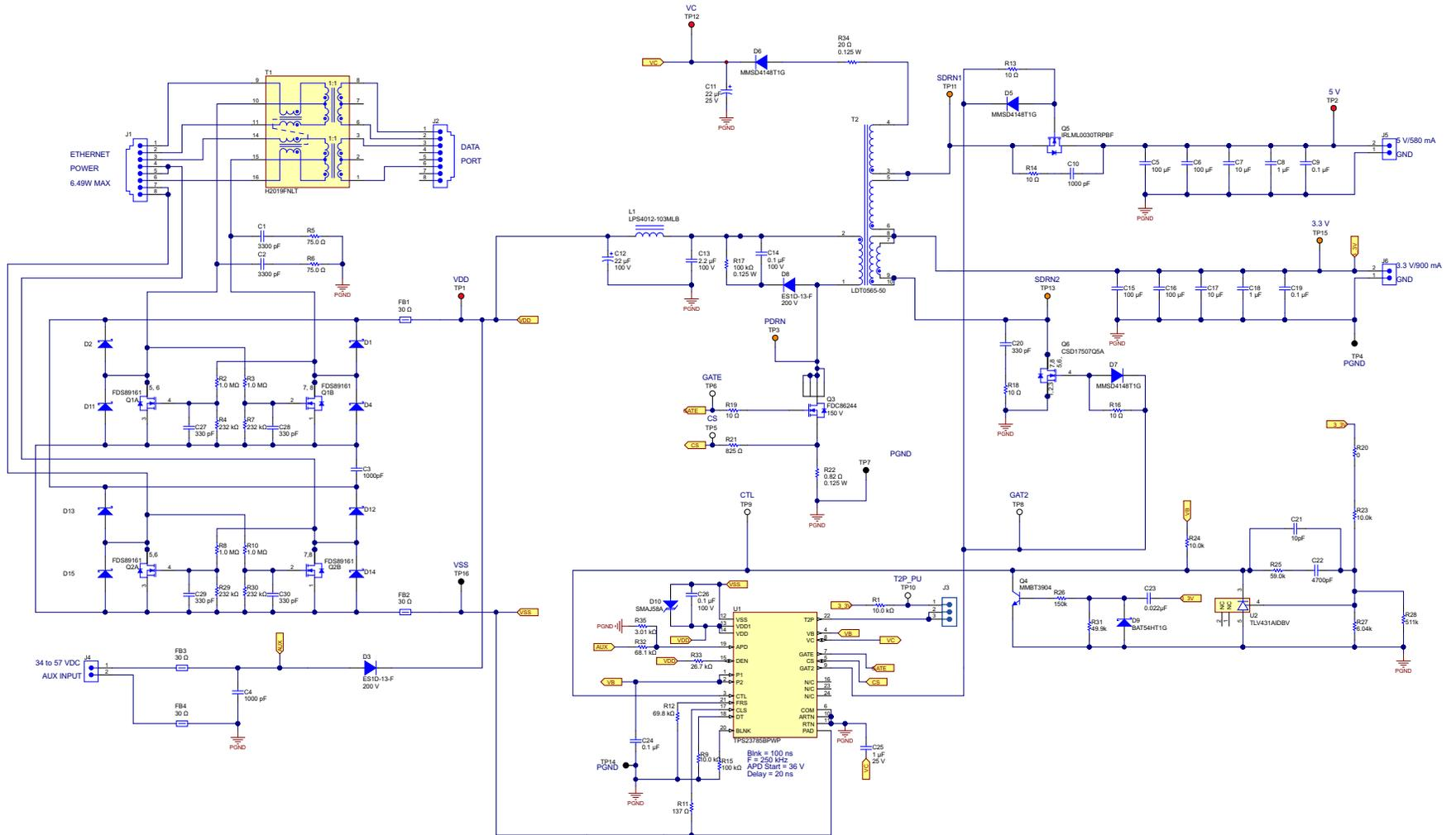
Figure 1. TPS23785BEVM-522 Schematic
