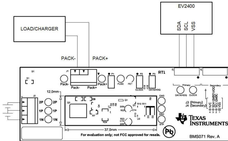
**Figure 1-1. BQ28Z620 Circuit Module Connection to Cells and System Load or Charger**
