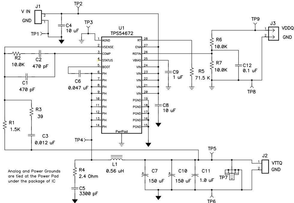
**Figure 8. Electrical Schematic of Evaluation Module TPS54672EVM-200**
