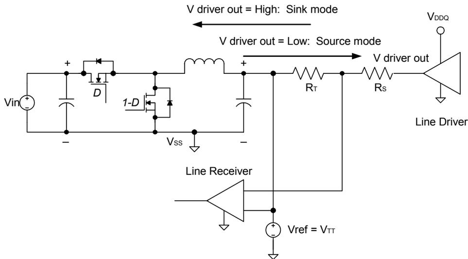
**Figure 1. Two Operating Modes of the Termination Voltage Regulator**
