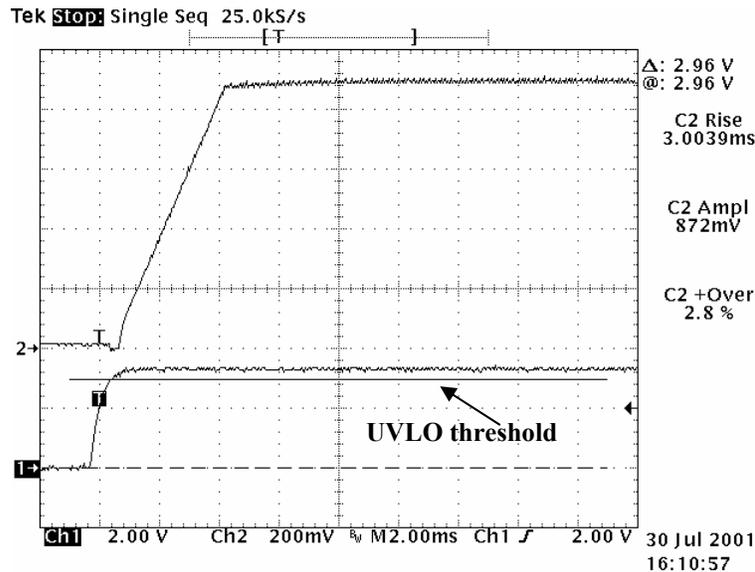
Figure 18. Start-Up Waveform by Applying the Input Voltage
