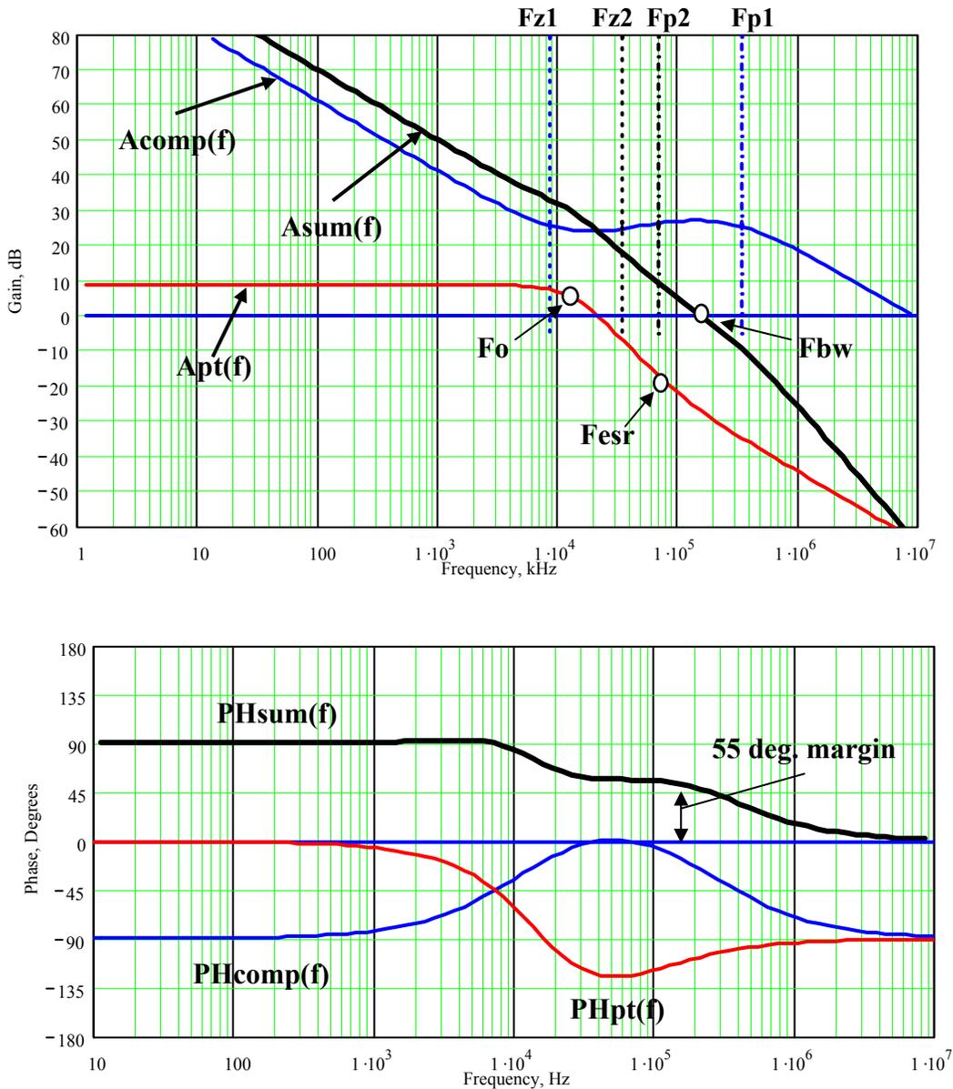
Figure 6. Overall Feedback Loop Bode Plots
