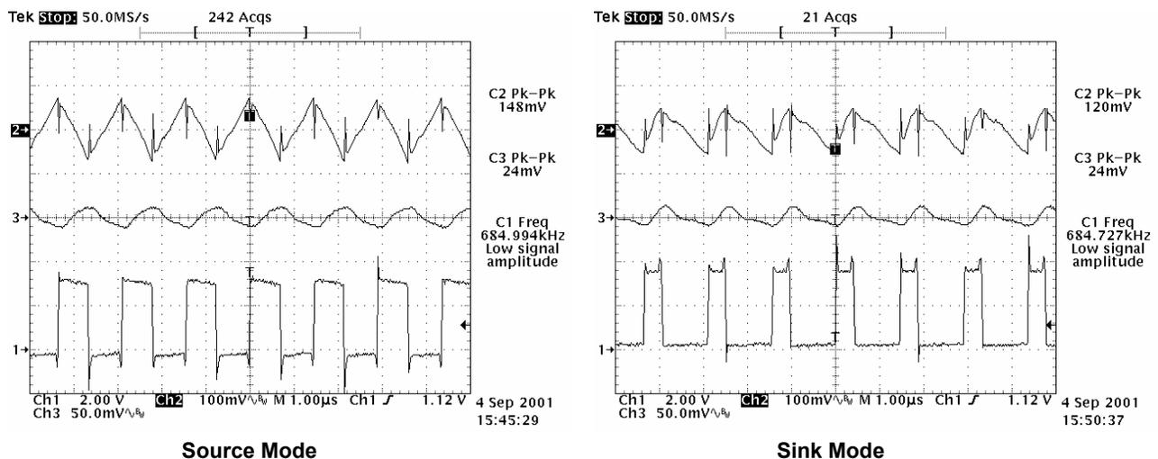
**Figure 9. Switching and Output/Input Ripple Waveforms**
