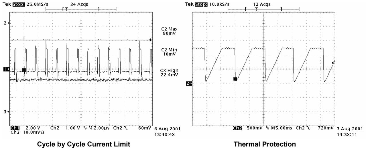
Figure 13. Two Types of Overcurrent Protection
