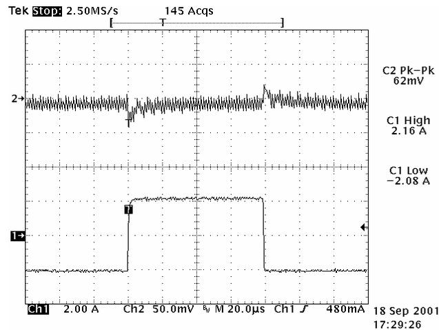
Figure 14. Load Current Transient Response
