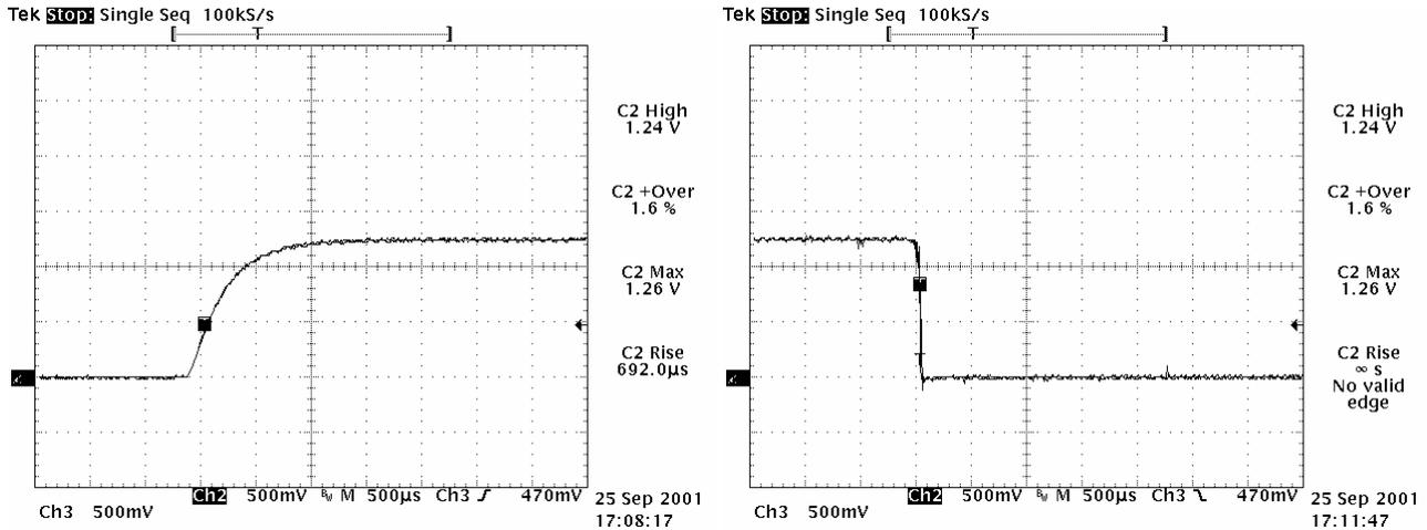
Figure 17. Output Voltage and Reference Input at Typical Slew-Rate
