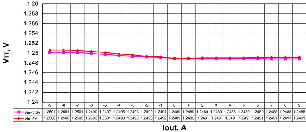
Figure 10. Line and Load Regulation
