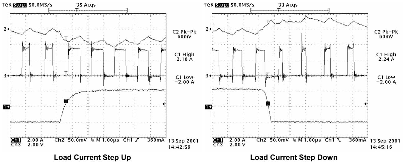
Figure 15. Expanded Load Current Transient Waveforms
