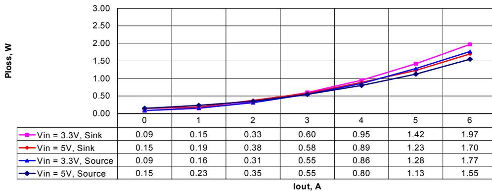
Figure 11. Power Losses Inside the Package
