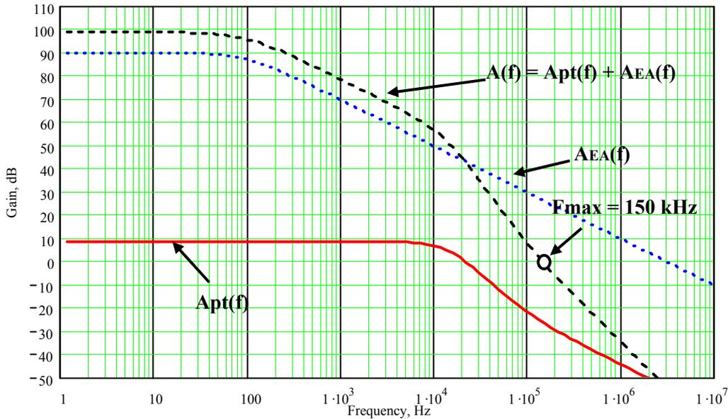
**Figure 4. Sum ( $A(f) = A_{pt}(f) + A_{EA}(f)$ ) of Gains of Regulator Output Stage and Error Amplifier**
