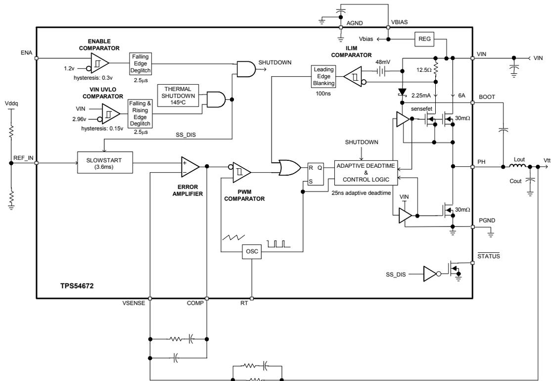
**Figure 2. TPS54672 Block Diagram**
