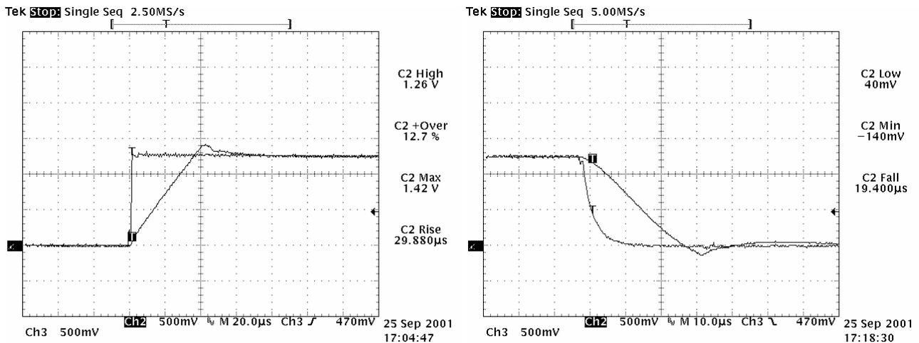
Figure 16. Output Voltage Response to the Reference Voltage Step Transient
