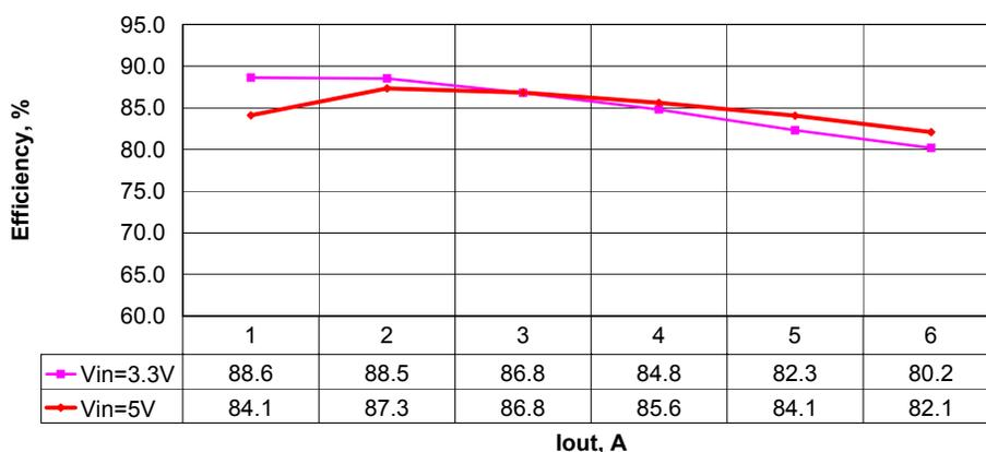
**Figure 12. Efficiency Curves at the Source Mode**
