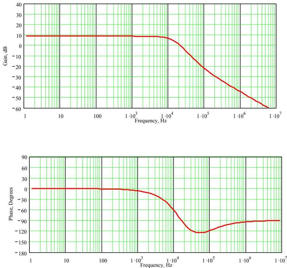
**Figure 3. Bode Plot of Output Stage of SWIFT Regulator Including PWM**
