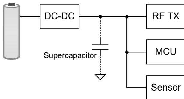
Figure 1. Power Tree of a Battery-Powered Wireless Sensor
