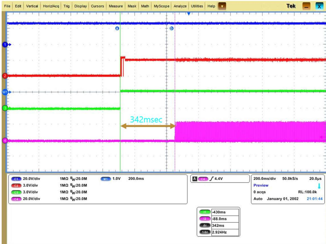
Ch1: 24 V, Ch2: SDA, Ch3: SPEED PIN Ch4: W PHASE VOLT of Motor
