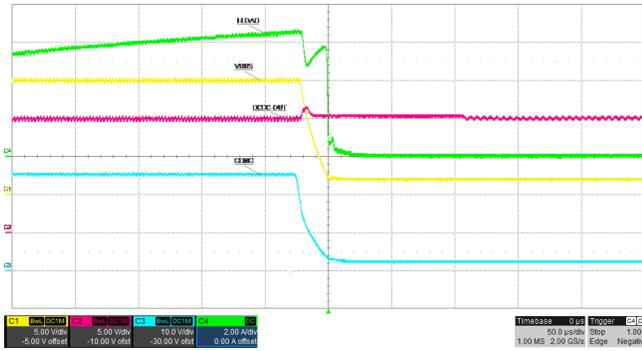
Figure 34. 8-A Soft Load Step Triggers 6.3-A OCP at 15 V
