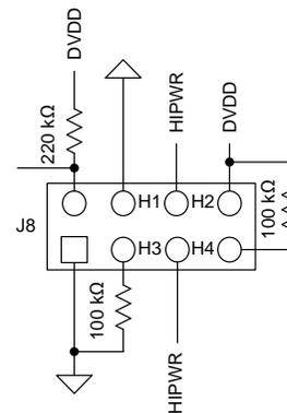
Figure 5. Voltage and J8 Current Select Header – J8
