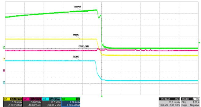
Figure 33. 8-A Soft Load Step Triggers 6.3-A OCP at 9 V
