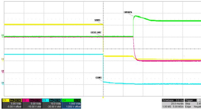
Figure 28. 5-A Transient Triggers OCP at 15 V
