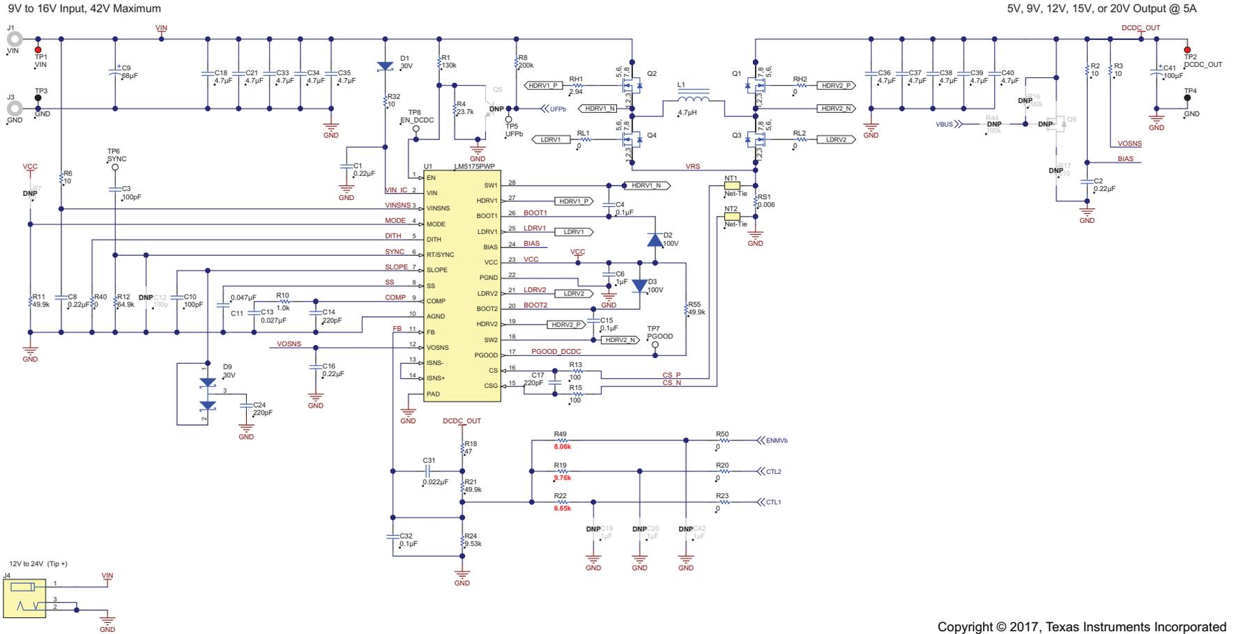
Figure 2. LM5175 Buck-Boost Power Supply
