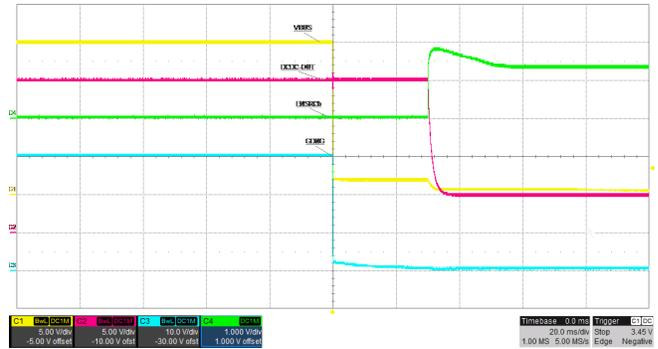
Figure 29. 5-A Transient Triggers OCP at 20 V
