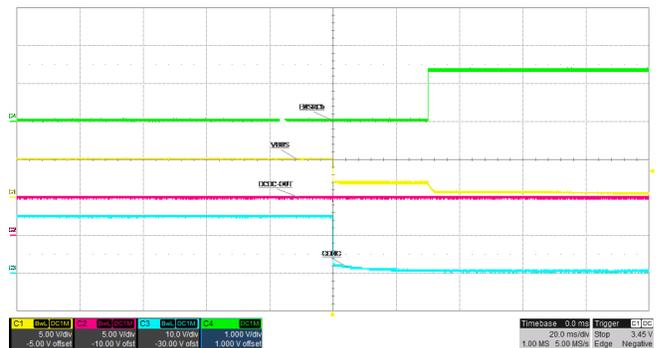
Figure 25. 5-A Transient Triggers OCP at 5 V
