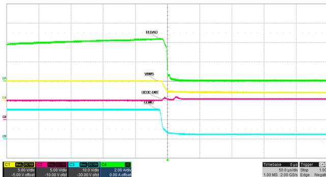
Figure 30. 5-A Soft Load Step Triggers 4.2-A OCP at 5 V
