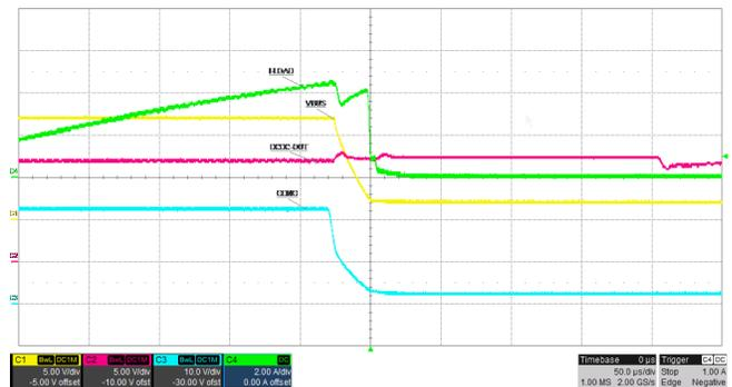
Figure 31. 5-A Soft Load Step Triggers 4.2-A OCP at 12 V
