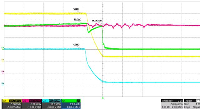
Figure 32. 5-A Soft Load Step Triggers 4.2-A OCP at 20 V
