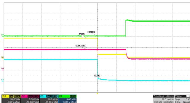
Figure 26. 5-A Transient Triggers OCP at 9 V
