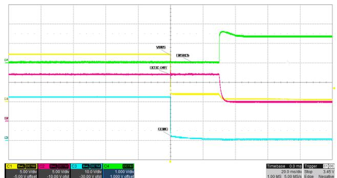
Figure 27. 5-A Transient Triggers OCP at 12 V
